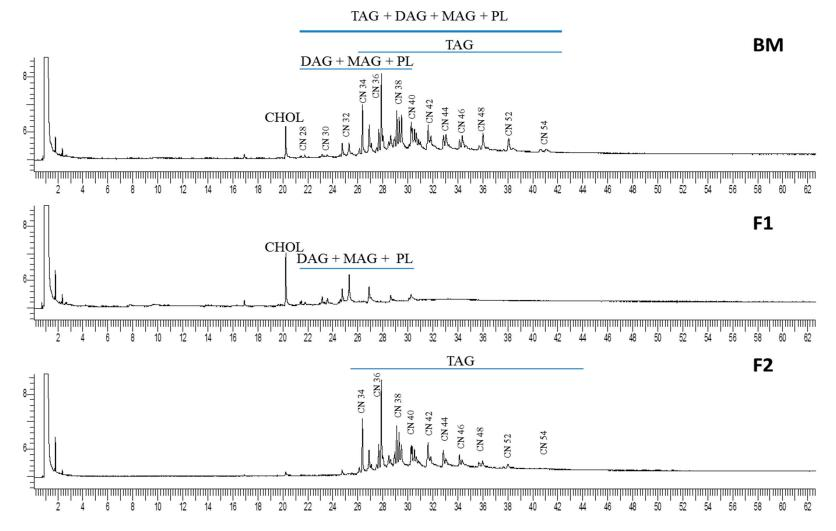
**Figure 2.** Chromatographic profile of lipid classes (DAG, diacylglycerides; CHOL, cholesterol; MAG, monoacylglycerides; PL, polar lipids) and molecular species of triacylglycerides (TAG) by carbon number (CN) of buttermilk (BM) and isolated fractions F1 and F2 determined by GC-FID.
