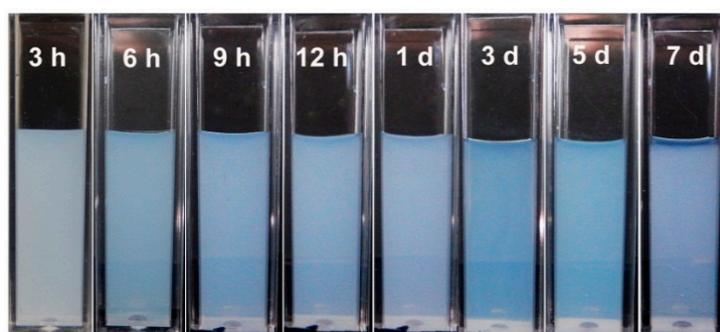
Figure 4. Photographs of Rod-CC NPs at a concentration of 1 mg/mL after standing still for 3, 6, 9, 12 h and 1, 3, 5, 7 day.
