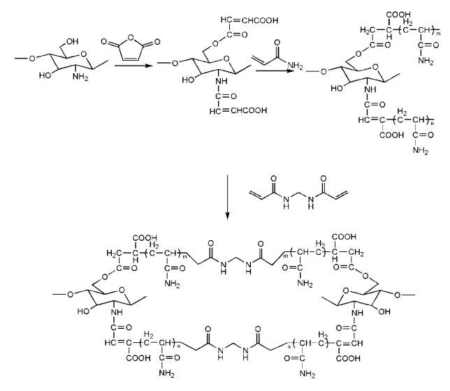
Figure 8. Cross-linking mechanism of maleic anhydride-modified chitosan and MBA.
