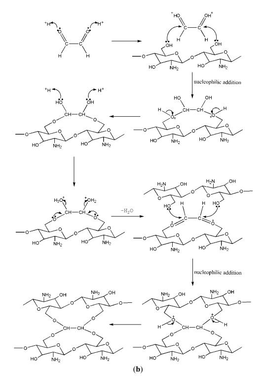
Figure 3. (a) Mechanism of primary reaction of chitosan and glyoxal; (b) Mechanism of secondary reaction of chitosan and glyoxal.
