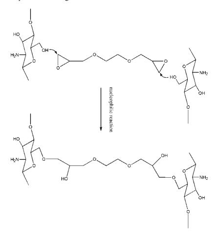
Figure 7. Cross-linking mechanism of chitosan and EGDE.
