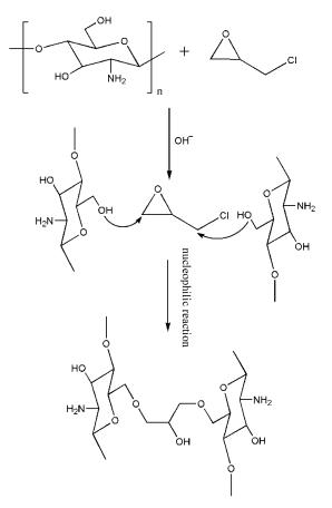
Figure 4. Cross-linking mechanism of chitosan and ECH under alkaline conditions.
