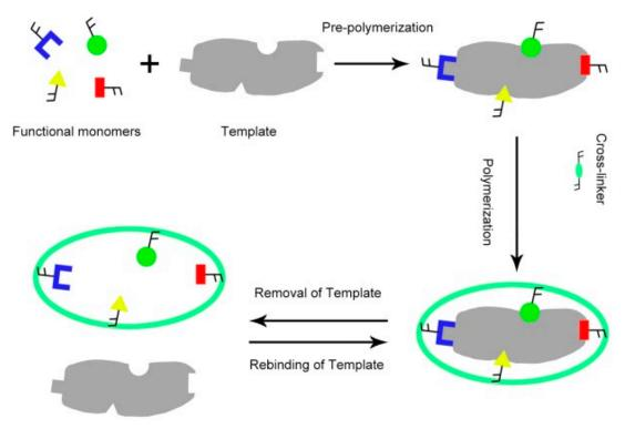
Figure 1. Schematic of molecular imprinting.
