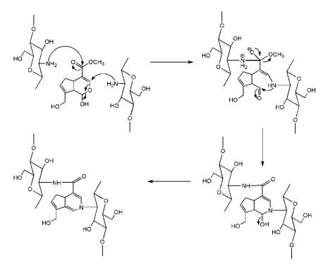
Figure 6. Cross-linking mechanism of chitosan and genipin.
