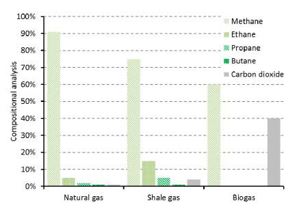
Figure 12. The composition of methane rich gases [117,198].
