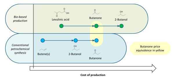
**Figure 4.** The effect of reversing the redox economy illustrated with 2-butanol. Relative costs of production have been estimated assuming a hypothetical scenario in which butanone prices are equivalent.
