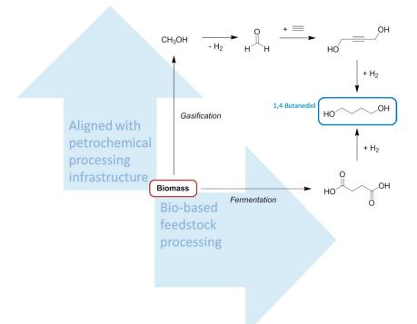
**Figure 3.** A comparison between the manufacturing processes of 1,4-butanediol from biomass. The solvent product is ringed in blue, the feedstock ringed in red.
