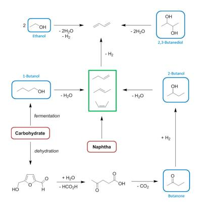
**Scheme 9.** Routes to butenes and 1,3-butadiene from bio-based alcohols. Key: red = feedstocks, green = key intermediate, blue = solvents.
