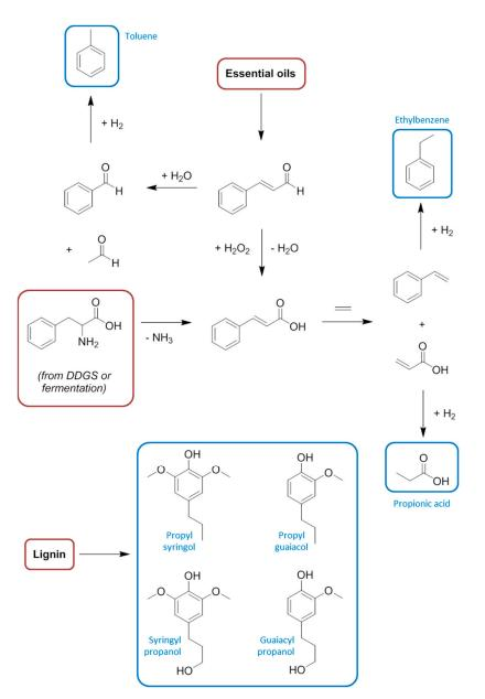
**Scheme 10.** Possible methods for the synthesis of some bio-based aromatic solvents. Key: red = feedstocks, blue = solvents.
