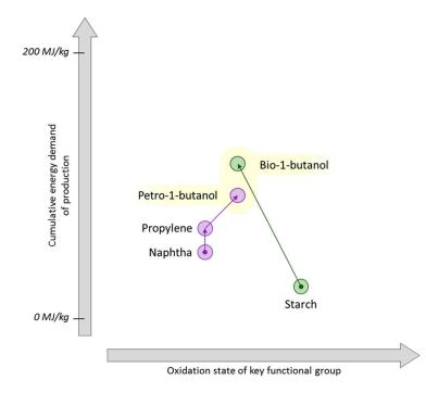
Figure 14. The cumulative energy demand of 1-butanol production.
