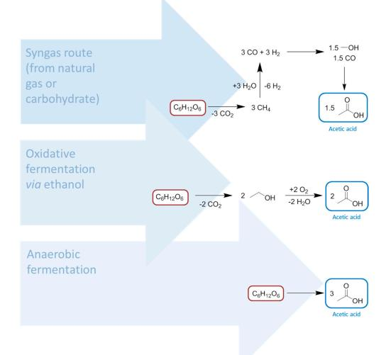
Figure 9. Stoichiometric reaction schemes for three approaches to the biosynthesis of acetic acid.
