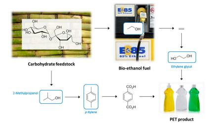
**Figure 1.** The interconnecting biofuel and bioplastic manufacturing industries and the solvent intermediates that result. Solvents are ringed in blue.
