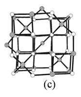
**Figure 1.** (a) Crystal packing of hematite, shaded circles represent Fe and unshaded circles represent O [23]; (b) Crystal packing of magnetite, dark large circles represent O, small light circles and small dark circles represent octahedral and tetrahedral coordinated Fe, respectively [24]; and (c) Crystal packing of maghemite, shaded circles represent Fe and unshaded circles represent O [23]. Reprinted with permission from reference [24].
