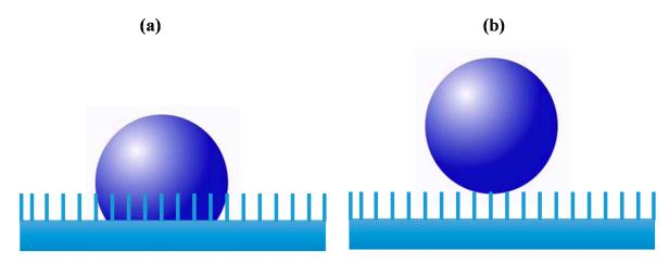
Figure 2. (a) Wendzel droplet (occurring when a water droplet merges with a surface) and (b) Cassie droplet (occurring when a water droplet is positioned on the surface) above nanosized pockets of ambient air.
