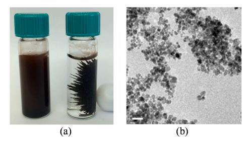
**Figure 6.** (a) Photograph of magnetite IONPs; left vial contains suspended IONPs while the Right vial contains IONPs subjected to a permanent magnet; and (b) TEM image of magnetite IONPs with 50 nm scale bar.
