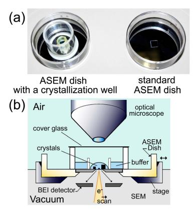
Here, we video-recorded copper sulfate crystallization in solution, utilizing the open sample holder of ASEM. Since the amount of backscattered electrons are related to atomic numbers and densities of atoms in the sample, we used heavy-metal staining to visualize lysozyme micro-crystals ( $2 \times 2.5 \mu m$ ), which are difficult to identify using OM. Finally, we directly observed non-stained crystals of three different proteins in crystallization buffers.
