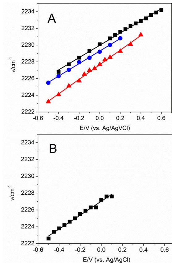
**Figure 5.** Changes in  $\text{C}\equiv\text{N}$  stretching band intensities with the electrode potential for Au/MBN (solid black squares), Au/thiophenol/MBN (solid blue circles), and Au/MHA/MBN (solid red triangles) obtained by SEIRA measurements, and Ag/MBN (hollow squares) obtained by SER measurements.
