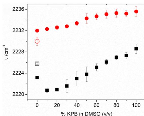
The nitrile stretching frequency of pure MBN SAMs on Ag and Au electrodes, both roughened on the 100-nm scale (see experimental section) was measured by SER and SEIRA spectroscopy, respectively. In the absence of any solvent, *i.e.*, for the SAM/air interfaces, the  $C\equiv N$  stretching frequency was determined to be  $2230.0 \pm 1.0$  and  $2225.8 \pm 0.2$   $\text{cm}^{-1}$  for Ag/MBN and Au/MBN,
