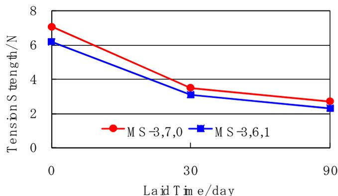
**Figure 11.** Tearing strength of mulch sheets laid on mandarin orange grove.
