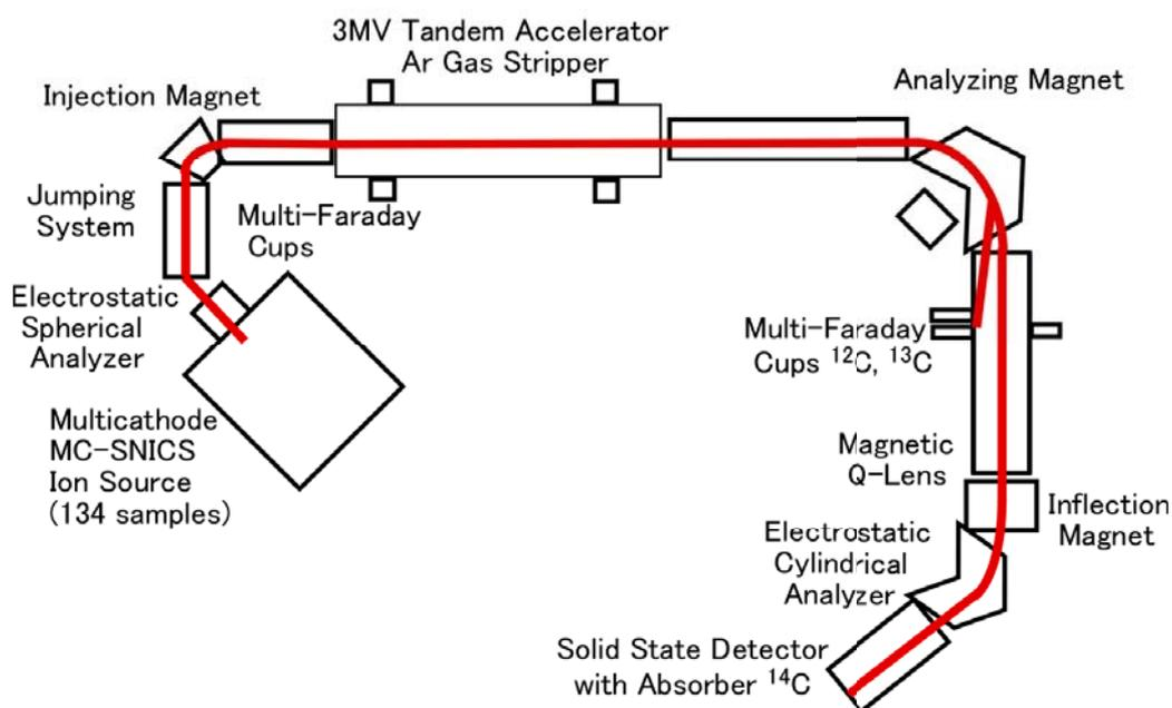
PLA and modified starch are biomass materials. When a product is used as a biobased material, it is important to measure the biomass carbon ratio. Recently, the accelerator mass spectroscopy (AMS) (Figure 2) measurement method for determining the biomass carbon ratio based on the American
