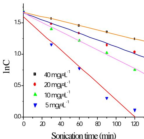
**Figure 4.** Degradation kinetics of methyl violet for different initial concentrations at 20°C.
