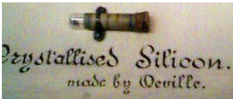
**Figure 3.** Sample of crystalline silicon by Deville.
