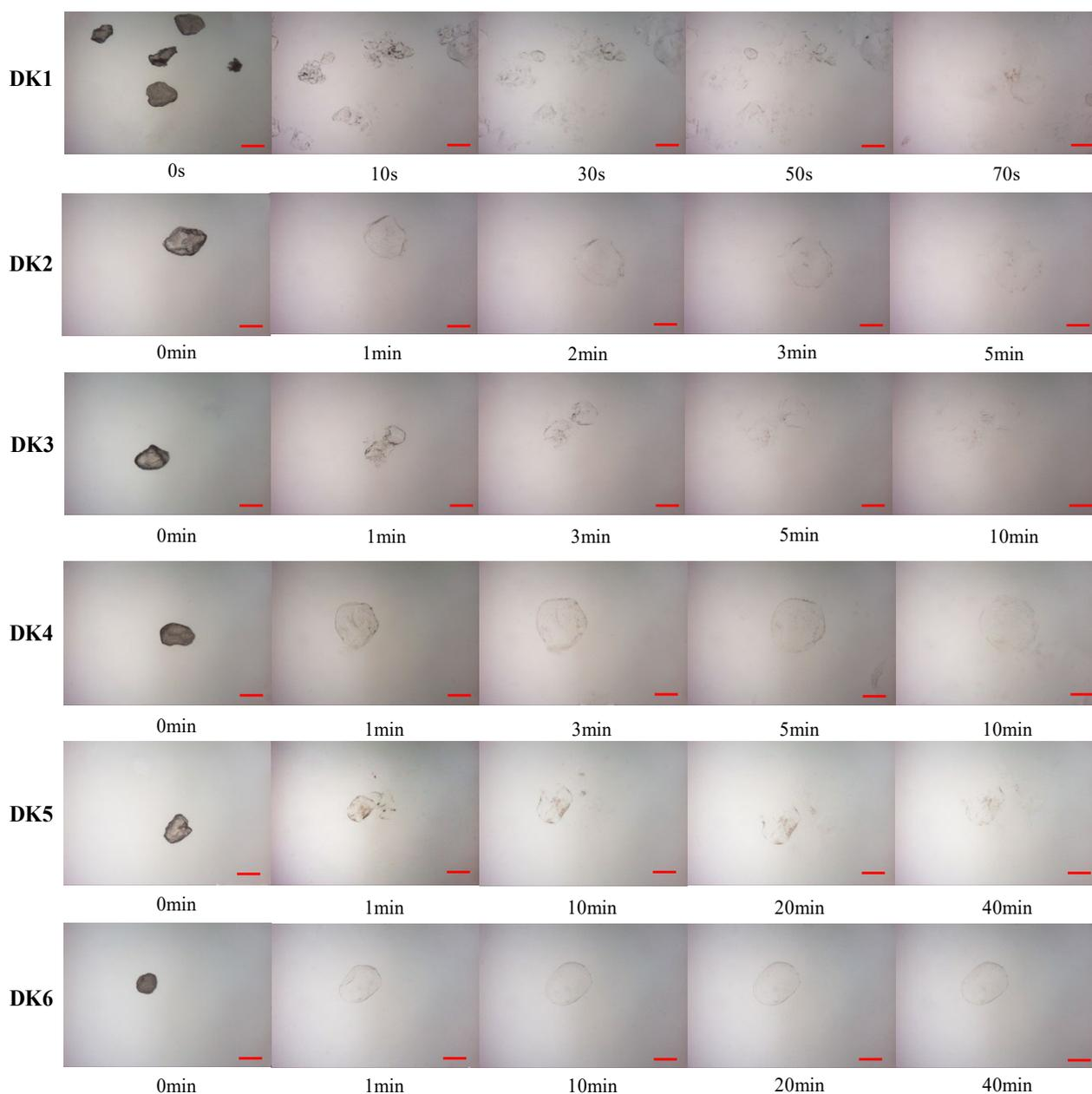
**Figure 3.** Dynamic swelling process of KGM with different DDs. The red bar in the graph represents 100  $\mu\text{m}$ .
