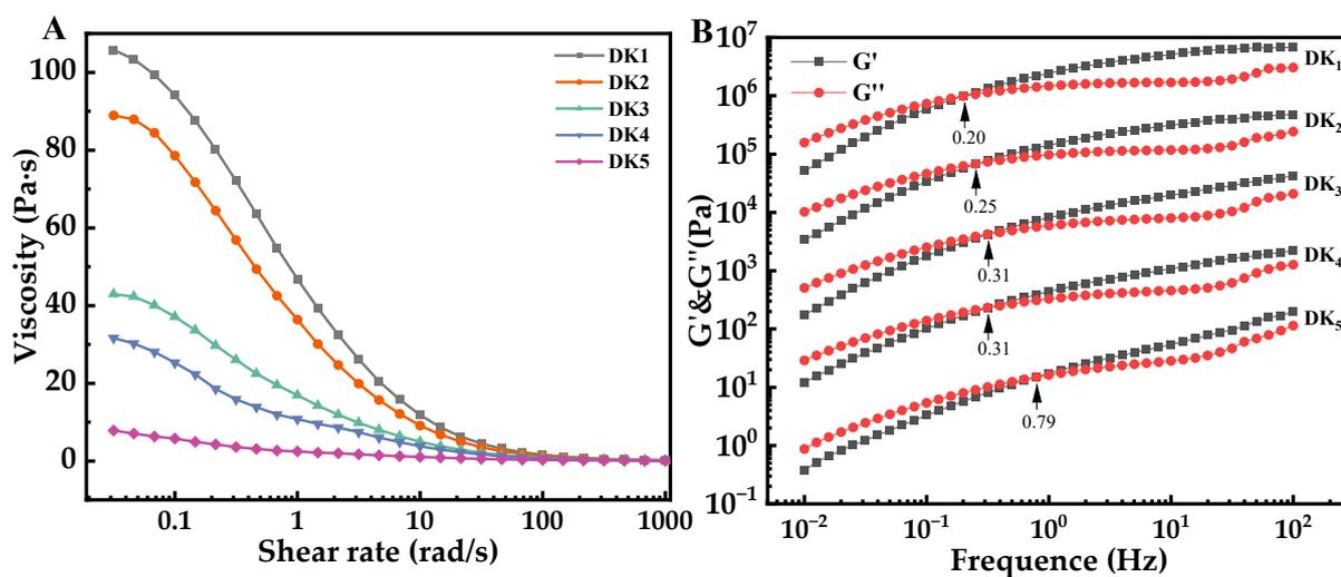
**Figure 5.** Steady-shear viscosity (A) and oscillation frequency sweep (B) of KGM sol with different degrees of deacetylation.
