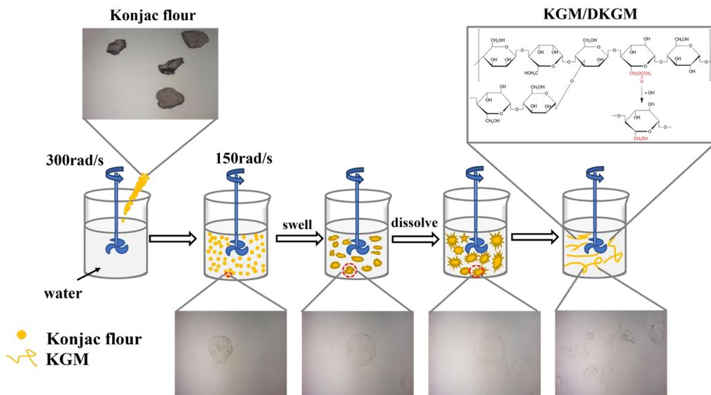
**Figure 2.** Schematic representation of KGM during swelling in water.
