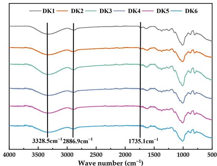
**Figure 1.** Infrared spectra of KGM with different DD. D1~D6 represent mixed konjac flour with different hydration rates.
