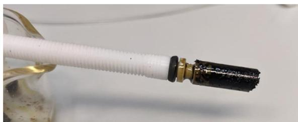
**Figure 1.** Picture of Aquivion  $\text{SO}_3\text{H}^{\text{®}}$  after its use under continuous flow conditions at  $140\text{ }^{\circ}\text{C}$ .
