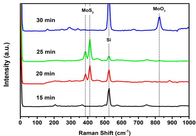
**Figure 2.** Raman spectra of various MoS<sub>2</sub> samples.
