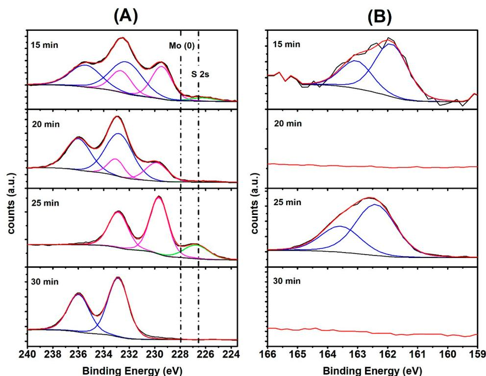
**Figure 3.** XPS synthesis of MoS<sub>2</sub>/rGO(n) at 15, 20, 25 and 30 min (A,B). Magenta lines of group A correspond to Mo(IV) and the blue ones are Mo(VI) (A). High-resolution XPS peak-shape of Mo 3d and S 2p, respectively.
