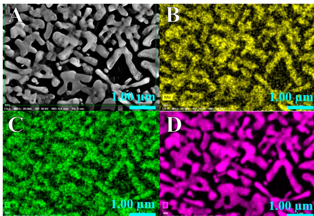
**Figure 1.** (A) SEM image and EDS element mapping of (B) Mo, (C) C and (D) S signal in MoS<sub>2</sub>/rGO(2).
