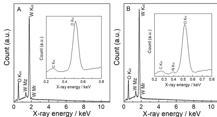
**Figure 2.** The EDS data of (A)  $\text{WO}_3-0$  and (B)  $\text{WO}_3-2.5$  in the range of 0–11 keV. (Insert) The magnified EDS data of  $\text{WO}_3-0$  and  $\text{WO}_3-2.5$  in the range of 0.2–0.8 keV, respectively.
