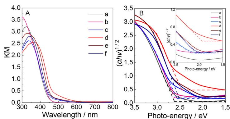
**Figure 6.** (A) UV-Visible DRS and (B) Tauc plots based on (a)  $WO_3-0$ , (b)  $WO_3-0.62$ , (c)  $WO_3-1.2$ , (d)  $WO_3-2.5$ , (e)  $WO_3-5$ , and (f)  $WO_3-7.5$ . Insets show the magnified spectra near the edges.
