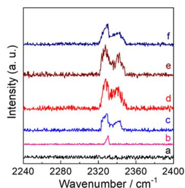
**Figure 5.** Raman spectra in the wavenumber region of  $2240\text{--}2400\text{ cm}^{-1}$  for (a)  $WO_3-0$ , (b)  $WO_3-0.62$ , (c)  $WO_3-1.2$ , (d)  $WO_3-2.5$ , (e)  $WO_3-5$ , and (f)  $WO_3-7.5$ , respectively.
