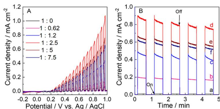
**Figure 9.** (A) Linear sweep voltammograms (LSV), and (B) Time course of the photocurrent at 0.68 V vs. Ag/AgCl (1.23 V vs. RHE) of the (a)  $\text{WO}_3-0$ , (b)  $\text{WO}_3-0.62$ , (c)  $\text{WO}_3-1.2$ , (d)  $\text{WO}_3-2.5$ , (e)  $\text{WO}_3-5$ , and (f)  $\text{WO}_3-7.5$  electrodes with visible-light irradiation chopped in a 0.1 M phosphate buffer solution of pH 6.0 with visible-light irradiation ( $\lambda > 450 \text{ nm}$ ,  $100 \text{ mW cm}^{-2}$ ).
