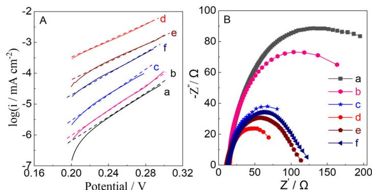
**Figure 12.** (A) Tafel plots and (B) Nyquist plots of (a)  $\text{WO}_3-0$ , (b)  $\text{WO}_3-0.62$ , (c)  $\text{WO}_3-1.2$ , (d)  $\text{WO}_3-2.5$ , (e)  $\text{WO}_3-5$ , and (f)  $\text{WO}_3-7.5$  electrodes for photoelectrocatalytic water oxidation in a 0.1 M phosphate buffer solution (pH = 6).
