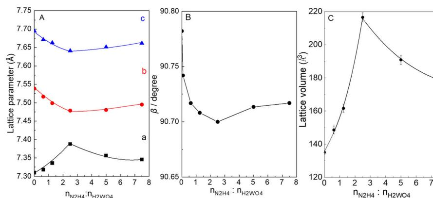
**Figure 4.** (A) Plots of lattice parameters of (a), (b), and (c) versus the addition of  $N_2H_4$ . (B) Plots of  $\beta$  versus the addition of  $N_2H_4$ , and (C) Lattice volumes of  $N_2$ -intercalated  $WO_3$  samples prepared with addition of  $N_2H_4$ . The lattice volume ( $V$ ) was calculated according to equation:  $V = abc(\sin\beta)$ ,  $\beta$  is the angle between  $a$  and  $c$ .
