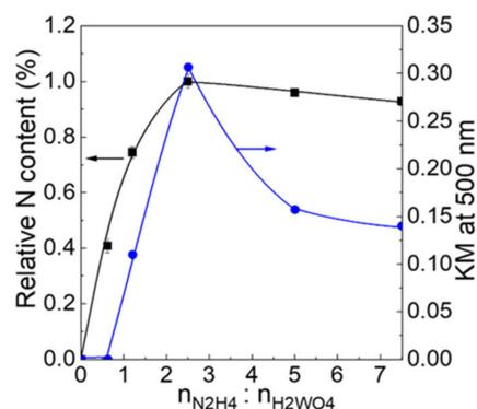
**Figure 7.** Relationship between the relative contents of N and  $n_{\text{H}_2\text{WO}_4}:n_{\text{N}_2\text{H}_4}$  ratio. The relative N contents were measured in EDS data and normalized by the highest contents for  $n_{\text{H}_2\text{WO}_4}:n_{\text{N}_2\text{H}_4}$  of 1:2.5.
