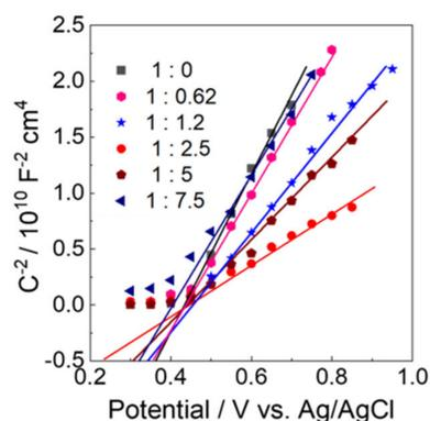
**Figure 8.** Mott-Schottky plots of (black)  $\text{WO}_3$ -0, (pink)  $\text{WO}_3$ -0.62, (blue)  $\text{WO}_3$ -1.2, (red)  $\text{WO}_3$ -2.5, (wine)  $\text{WO}_3$ -5, and (navy)  $\text{WO}_3$ -7.5 electrodes in a 0.1 M phosphate buffer solution of pH 6.0. frequency, 0.1 Hz; amplitude potential, 10 mV.
