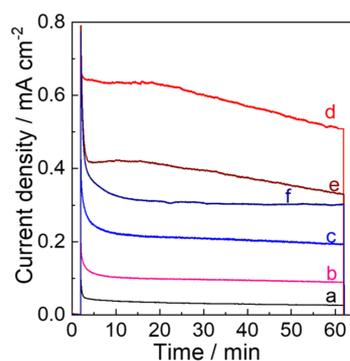
**Figure 11.** Photocurrent density versus time profiles during PEC water oxidation in a 0.1 M phosphate buffer solution of pH 6.0 at 0.68 V vs. Ag/AgCl (1.23 V vs. RHE) upon visible-light irradiation ( $\lambda > 450$  nm,  $100 \text{ mWcm}^{-2}$ ) using (a)  $WO_3-0$ , (b)  $WO_3-0.62$ , (c)  $WO_3-1.2$ , (d)  $WO_3-2.5$ , (e)  $WO_3-5$ , and (f)  $WO_3-7.5$  electrodes.
