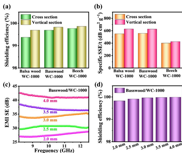
**Figure 6.** (a) EMI shielding efficiencies and (b) SSE/t values of WC-1000 (balsa wood, basswood and beech) under different sections. (c) EMI SE<sub>T</sub> and (d) EMI shielding efficiencies of WC-1000 of basswood at different thicknesses.
