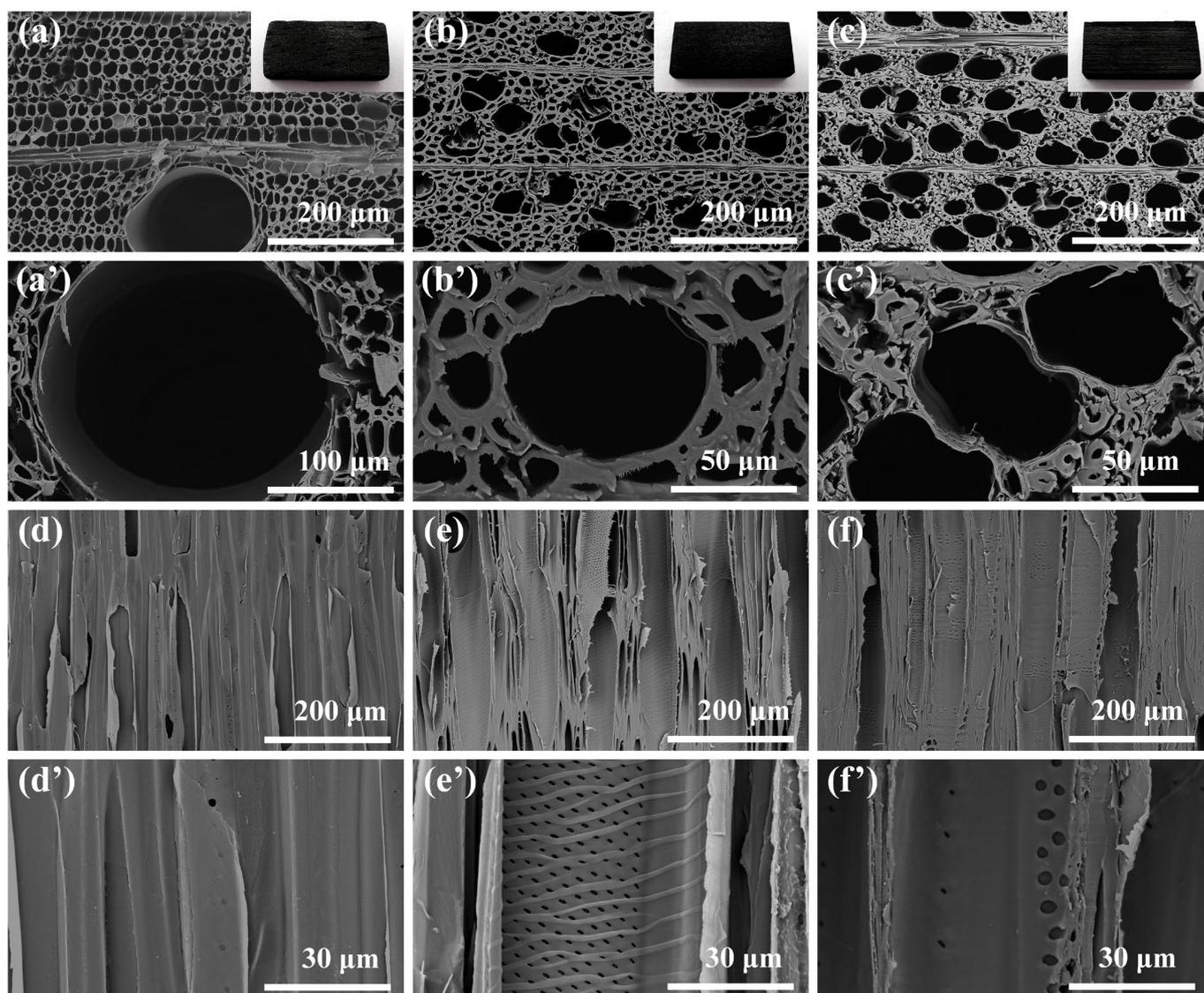
**Figure 2.** SEM images and pictures of balsawood-derived carbon (a,a'), basswood-derived carbon (b,b') and beech-derived carbon (c,c') in the cross-section, and SEM images of balsawood-derived carbon (d,d'), basswood-derived carbon (e,e') and beech-derived carbon (f,f') in the vertical-section.
