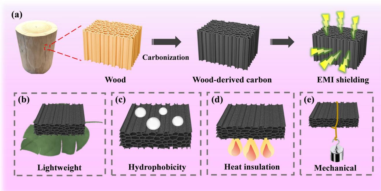
**Figure 1.** (a) Schematic of the preparation of WC for EMI shielding with (b) lightweight, (c) hydrophobicity, (d) heat insulation and (e) mechanical properties.
