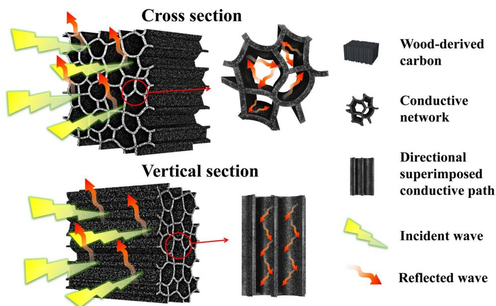
**Figure 7.** Schematic diagram of EMI shielding mechanism of WC materials.
