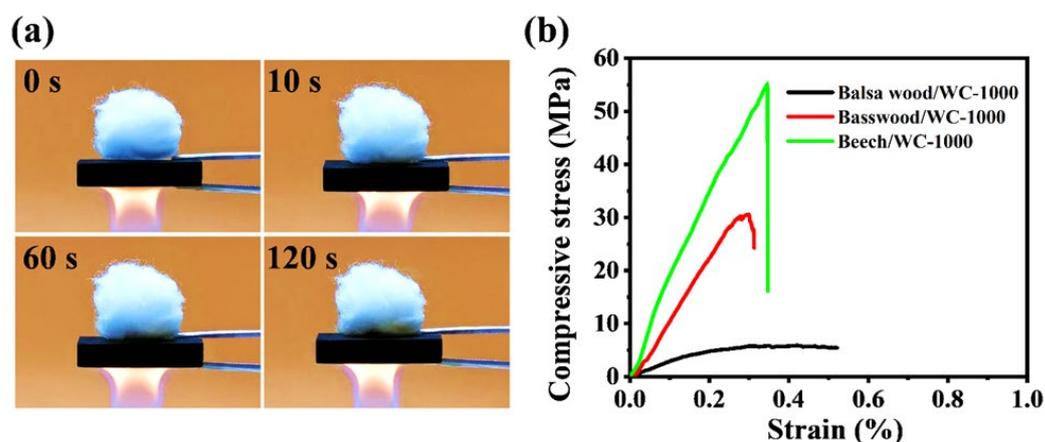
**Figure 8.** (a) Photos of basswood-derived carbon after combustion. (b) Compressive stress–strain curves of WC-1000 (balsa wood, basswood and beech).
