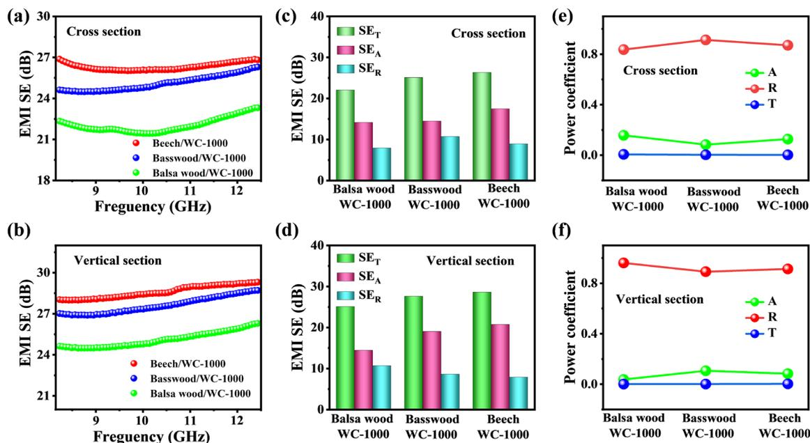
**Figure 5.** (a,b) EMI  $SE_T$ ; (c,d) comparison of the average  $SE_T$ ,  $SE_A$  and  $SE_R$  values; and (e,f) the A, R and T values of WC-1000 (balsa wood, basswood and beech) under different sections.
