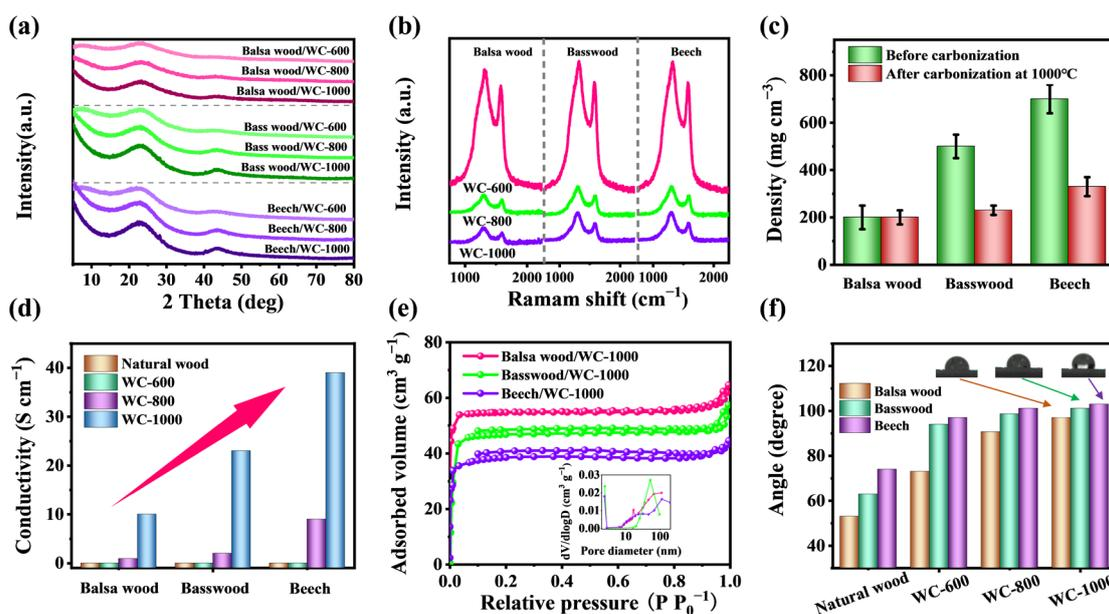
**Figure 3.** (a) XRD spectra and (b) Raman spectra of WC-600, CWF-800 and CWF-1000 of balsa wood, basswood and beech. (c) Densities and (d) electrical conductivities of samples. (e) N<sub>2</sub> adsorption-desorption isotherms and pore size distributions. (f) The contact angles of samples.
