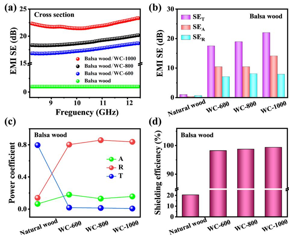
**Figure 4.** (a) EMI  $SE_T$ ; (b) comparison of the average  $SE_T$ ,  $SE_A$  and  $SE_R$  values; (c) the A, R and T values and (d) EMI shielding efficiencies of natural wood, WC-600, WC-800 and WC-1000 of balsa wood.
