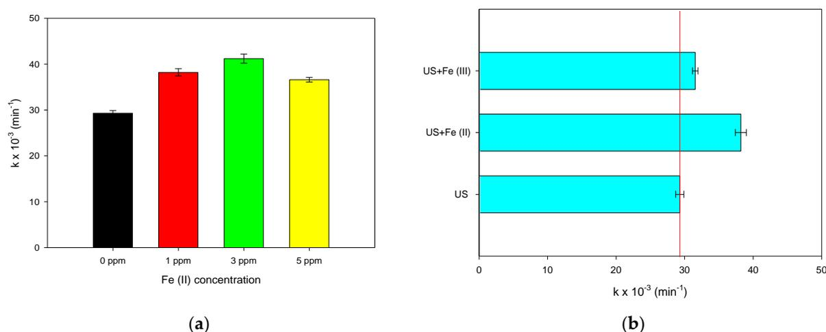
**Figure 3.** Homogeneous sono-Fenton for degrading MO as the probe compound. (a) Effect of iron (II) ions concentration; (b) Effect of the iron species (II or III, at 1 ppm ( $\text{mg L}^{-1}$ )). Experimental conditions:  $f$ : 375 kHz,  $P$ : 34.4 W,  $[\text{MO}]_{\text{initial}}$ :  $30.6 \mu\text{mol L}^{-1}$ ,  $\text{pH}_{\text{initial}}$ : 5.6, and  $V$ : 250 mL.
