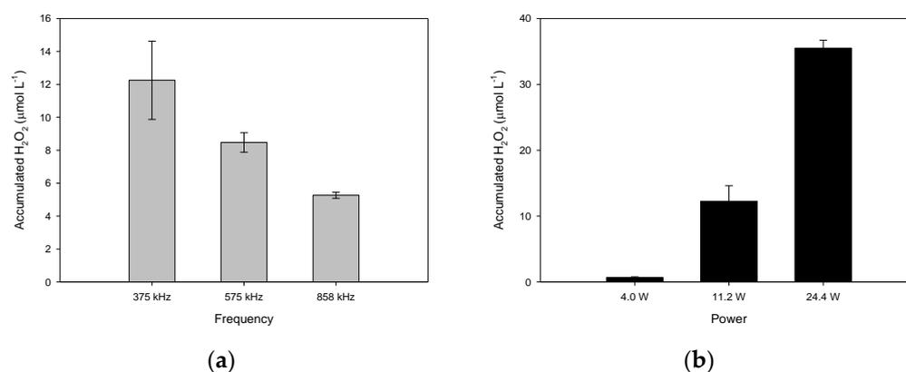
**Figure 1.** Capability of the ultrasound reactor to produce  $\text{H}_2\text{O}_2$  in distilled water at 20 min of sonication. (a) Effect of the ultrasound frequency (V: 250 mL, P: 11.2 W); (b) Effect of ultrasound power (V: 250 mL, f: 375 kHz).
