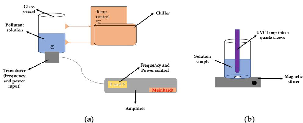
**Figure 8.** Scheme of the experimental setups. (a) Ultrasound reactor for the sono-Fenton process, in this reactor, frequency and power can be adjusted. (b) Reactor for the photo-treatment.
