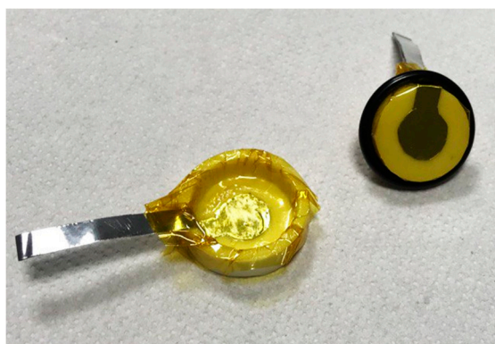
Figure S4. The modified mold used for poling during the cross-linking. Each part is equipped with an aluminum electrode and covered with a dielectric film. The positive mold has an O-ring tighten around to control the thickness of the final composite.
