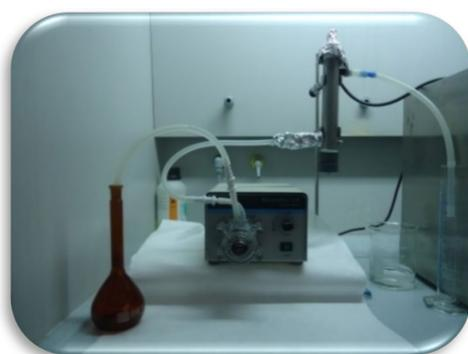
**Figure 1.** Semi-continuous reactor used for the degradation of terbuthylazine in ultrapure water, groundwater and water from the Gaditana area.
