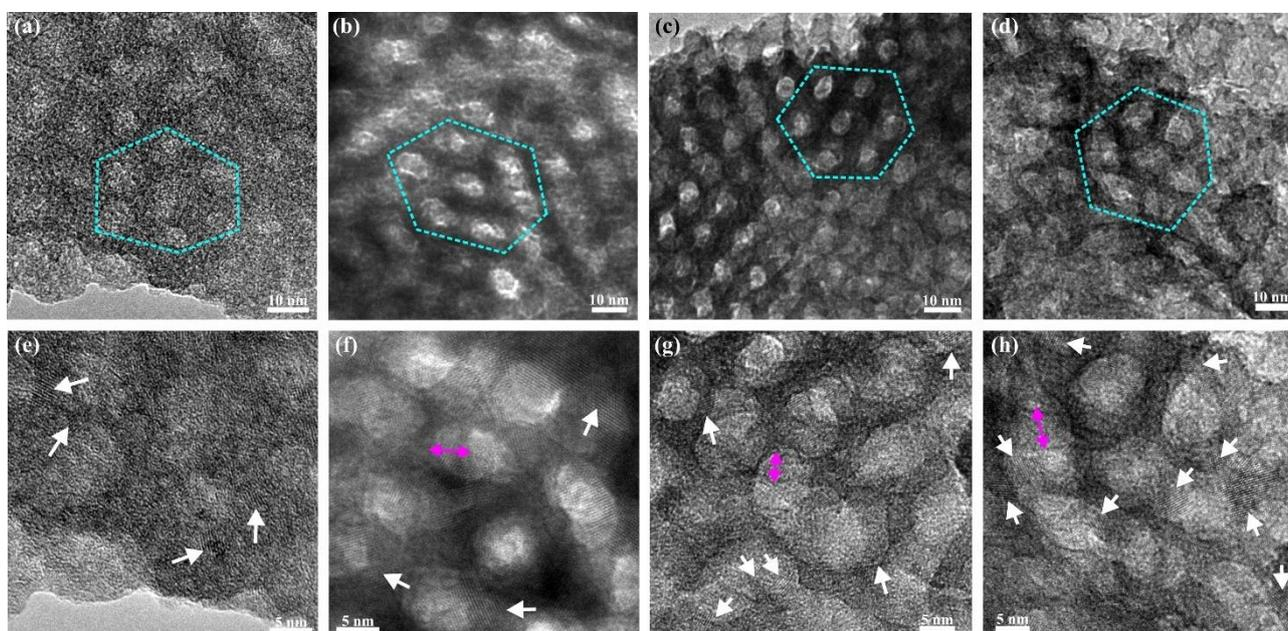
**Figure 3.** BF TEM images of mesostructured titania with synthesis time 3 h, before template removal (a), and after template removal with synthesis times of 3 h (b), 6 h (c), and 24 h (d). The hexagonal order of the pores has been outlined with cyan dotted lines. (e–h) HRTEM images of samples (a–d), respectively, in which some of the anatase crystalline areas are highlighted with white arrows. Magenta double arrows denote the shadowing of pores due to the inclined viewing direction.
