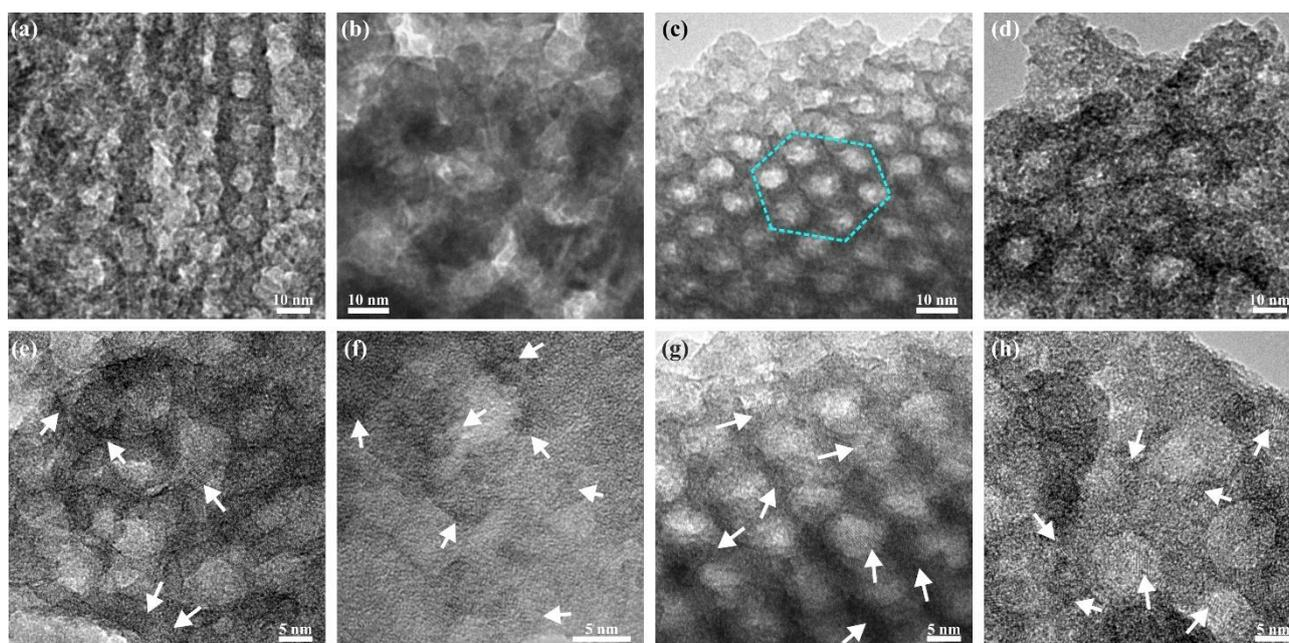
**Figure 4.** (HR)TEM images of mesoporous titania with 3 h synthesis time, deposited with 60 s spray coating and aged at 75% RH for (a,e) 1 h, (b,f) 48 h, (c,g) 72 h, and (d,h) 120 h. A hexagonal pore order was achieved for the sample aged for 72 h and is outlined with dotted cyan line (c). White arrows indicate some of the anatase crystallites.
