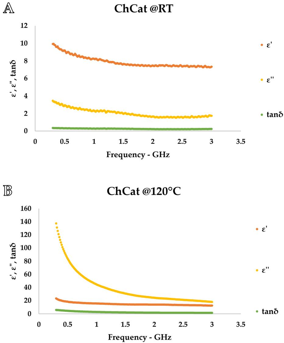
**Figure S6:** ChCat dielectric properties. Irradiation frequency range: 0.3-3 GHz. Irradiation temperature: A. RT; B. 120 °C. Measurements were performed according to Paragraph 3.3 in the Experimental Section.
