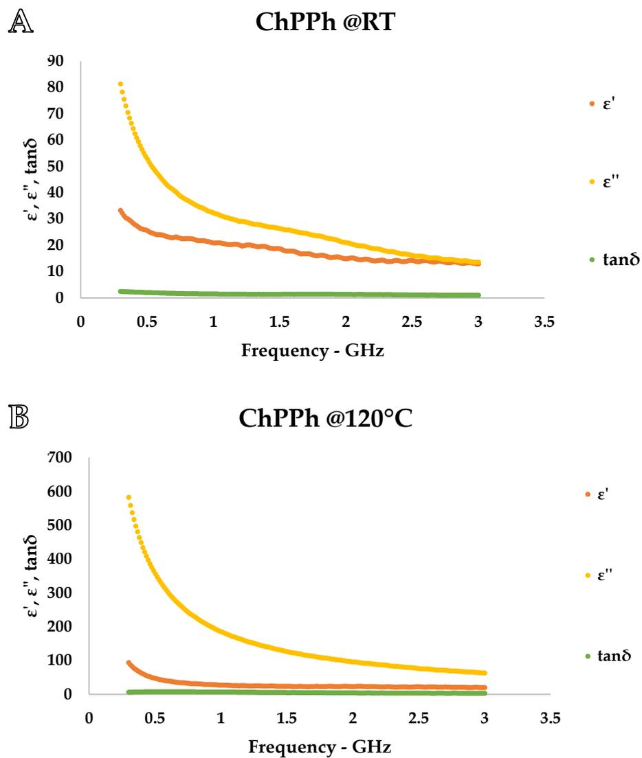
**Figure S11:** ChPPh dielectric properties. Irradiation frequency range: 0.3-3 GHz. Irradiation temperature: A. RT; B. 120 °C. Measurements were performed according to Paragraph 3.3 in the Experimental Section.
