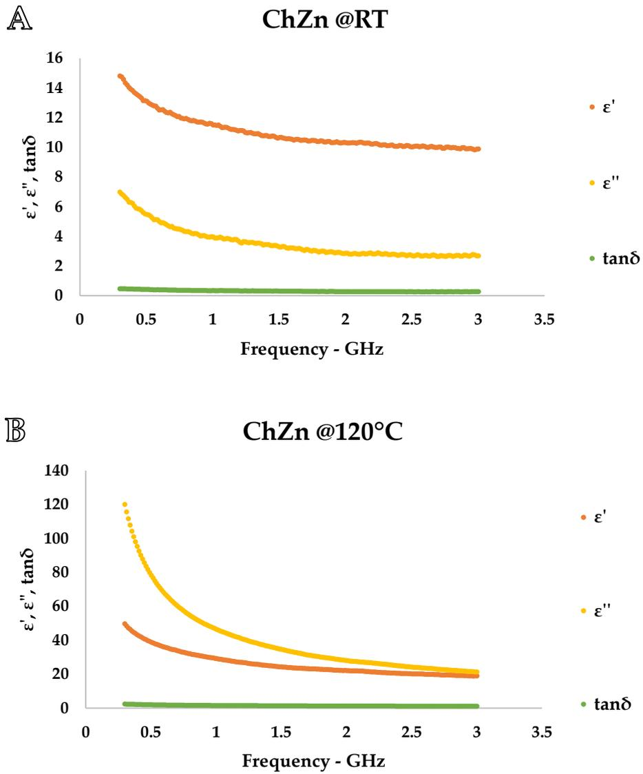
**Figure S4:** ChZn dielectric properties. Irradiation frequency range: 0.3-3 GHz. Irradiation temperature: A. RT; B. 120 °C. Measurements were performed according to Paragraph 3.3 in the Experimental Section.
