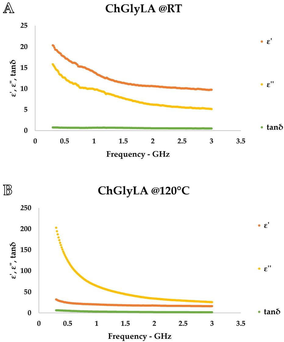
**Figure S3:** ChGlyLA dielectric properties. Irradiation frequency range: 0.3-3 GHz. Irradiation temperature: A. RT; B. 120 °C. Measurements were performed according to Paragraph 3.3 in the Experimental Section.
