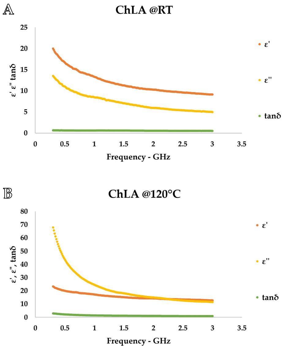
**Figure S1:** ChLA dielectric properties. Irradiation frequency range: 0.3-3 GHz. Irradiation temperature: A. RT; B. 120 °C. Measurements were performed according to Paragraph 3.3 in the Experimental Section.
