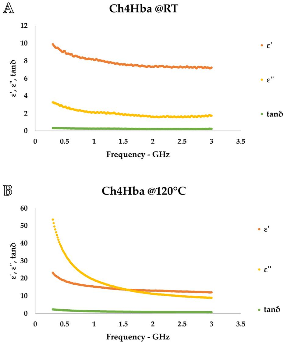
**Figure S5:** Ch4Hba dielectric properties. Irradiation frequency range: 0.3-3 GHz. Irradiation temperature: A. RT; B. 120 °C. Measurements were performed according to Paragraph 3.3 in the Experimental Section.
