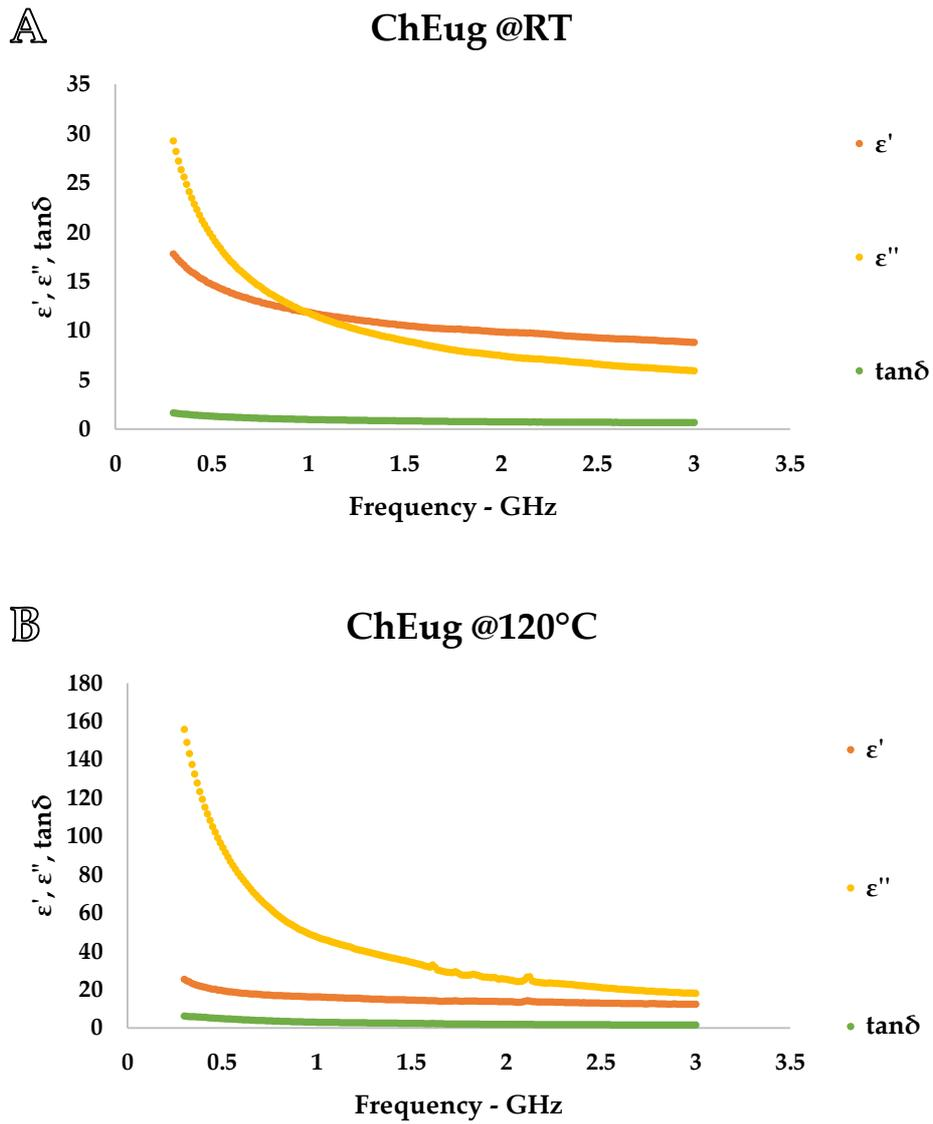
**Figure S7:** ChEug dielectric properties. Irradiation frequency range: 0.3-3 GHz. Irradiation temperature: A. RT; B. 120 °C. Measurements were performed according to Paragraph 3.3 in the Experimental Section.
