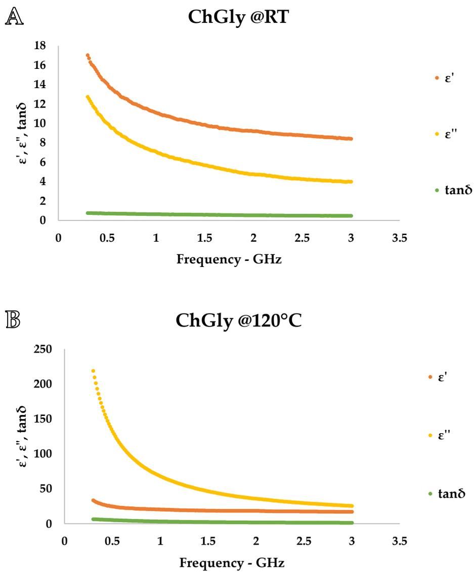
**Figure S2:** ChGly dielectric properties. Irradiation frequency range: 0.3-3 GHz. Irradiation temperature: A. RT; B. 120 °C. Measurements were performed according to Paragraph 3.3 in the Experimental Section.
