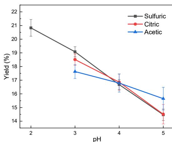
Figure 1. Yield of the isolated lignin in various pH and acid types.
