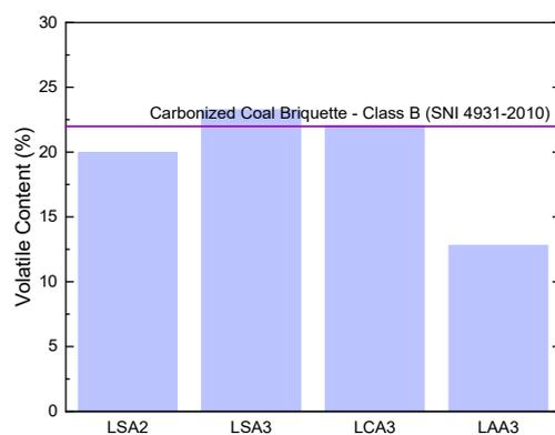
**Figure 4.** Volatile content of lignin LSA2, LSA3, LCA3, and LAA3 with carbonized coal briquette SNI (4931–2010).
