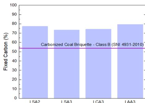
**Figure 6.** Fixed carbon of LS2, LS3, LAS3, and LAA3 samples compared to the carbonized coal briquette SNI 4931–2010.
