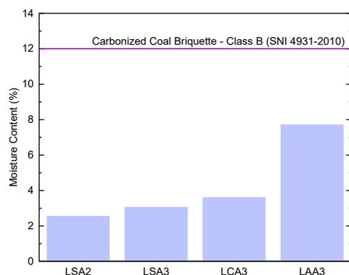
**Figure 3.** Moisture content of lignin LSA2, LSA3, LCA3, and LAA3 compared to carbonized coal briquette from the SNI 4931–2010 requirement.
