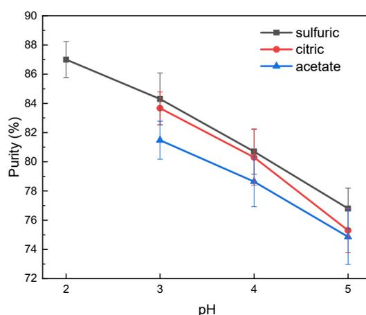
Figure 2. The purity of isolated lignin in various pH and acid types.
