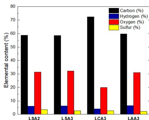
**Figure 8.** Effect of Acid Type on Ultimate Analysis of LSA2, LSA3, LCA3, and LAA3.
