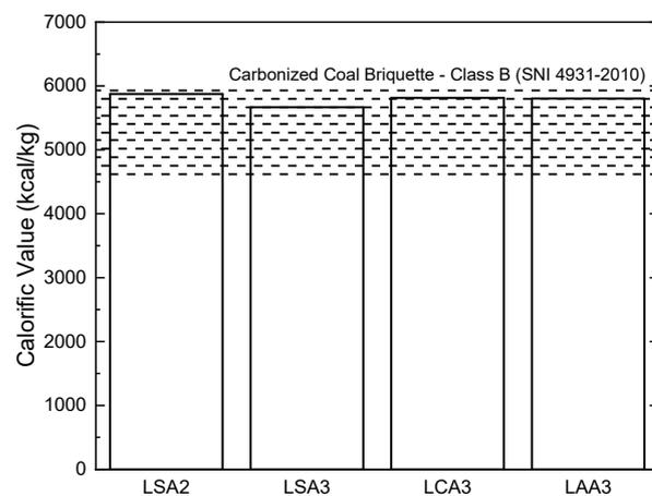
**Figure 11.** Calorific Value of the Resultant Lignin Briquettes.
