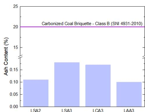
**Figure 5.** Ash content of the lignin LS2, LS3, LCA3, and LAA3 compared to the carbonized coal briquette SNI 4931–2010.
