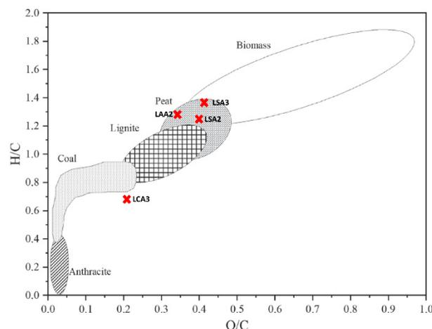
**Figure 10.** Position of the resultant Briquette on the Van Kravlen diagram (adapted and modified from [31]).
