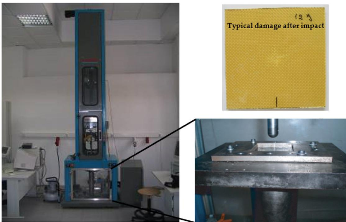
**Figure 2.** Details of the drop weight testing machine and a specimen with typical damage obtained after an impact with 12 J and immediately before immersion in hostile solutions.
