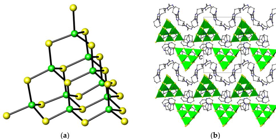
**Figure 1.** (a) The T3 supertetrahedral cluster found in  $[\text{C}_9\text{H}_{17}\text{N}_2]_6[\text{Ga}_{10}\text{S}_{16}(\text{SH})_4]$ . Color key: green spheres, Ga; yellow spheres, S. (b) View of the crystal structure along the  $a$ -axis. Unit cell is shown. Color key:  $\text{GaS}_4$ , green tetrahedra; yellow spheres, S; blue spheres, N; grey spheres, C. H atoms have been omitted for clarity.
