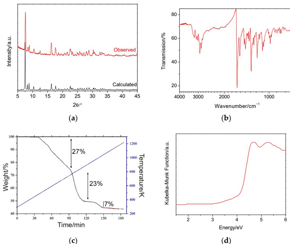
**Figure 2.** (a) Powder X-ray diffraction data collected for ground crystals of  $[\text{C}_9\text{H}_{17}\text{N}_2]_6[\text{Ga}_{10}\text{S}_{16}(\text{SH})_4]$ . (b) FT-IR data. (c) Thermogravimetric analysis data, collected under air. The temperature is given by the blue line. (d) UV-Vis diffuse reflectance data.
