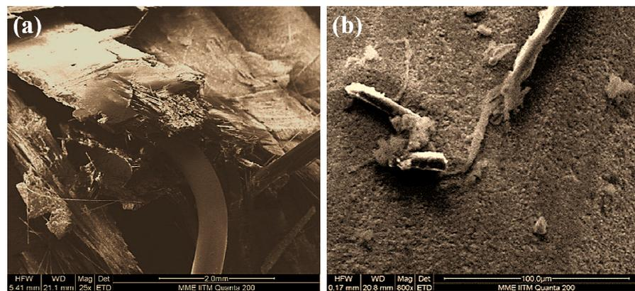
**Figure 7.** SEM micrograph of (a) SMA/matrix debonding failure mode, (b) interaction of SMA wire with GFRP and matrix, after impact.
