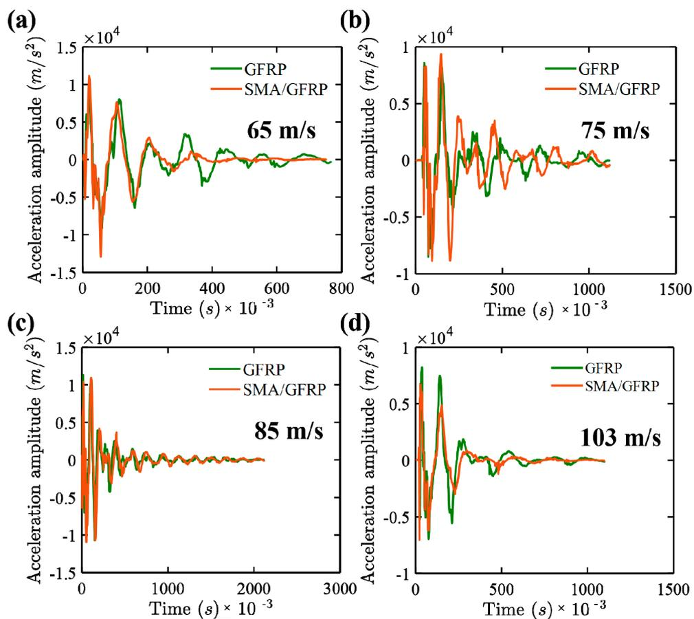
**Figure 8.** Acceleration–time response for the GFRP and SMA/GFRP specimens at different impact velocities (a) 65 m/s, (b) 75 m/s, (c) 85 m/s, and (d) 103 m/s (zoomed version of this plot is provided in Figure S1—Supplementary Materials).
