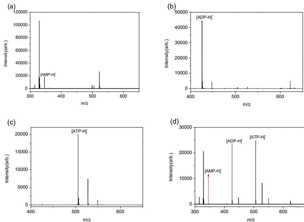
Fig S7. MALDI mass spectra of (a) AMP (1nmol) (b) ADP (1nmol) (c) ATP (1nmol) (d) AMP:ADP:ATP = 1:1:1 (0.33nmol for each one) with DHBA IL in negative reflectron mode. The molar matrix-to-analyte ratio was approximately 500:1. Laser intensity was 95%. 1000 laser shots randomly distributed in 20 different positions.
