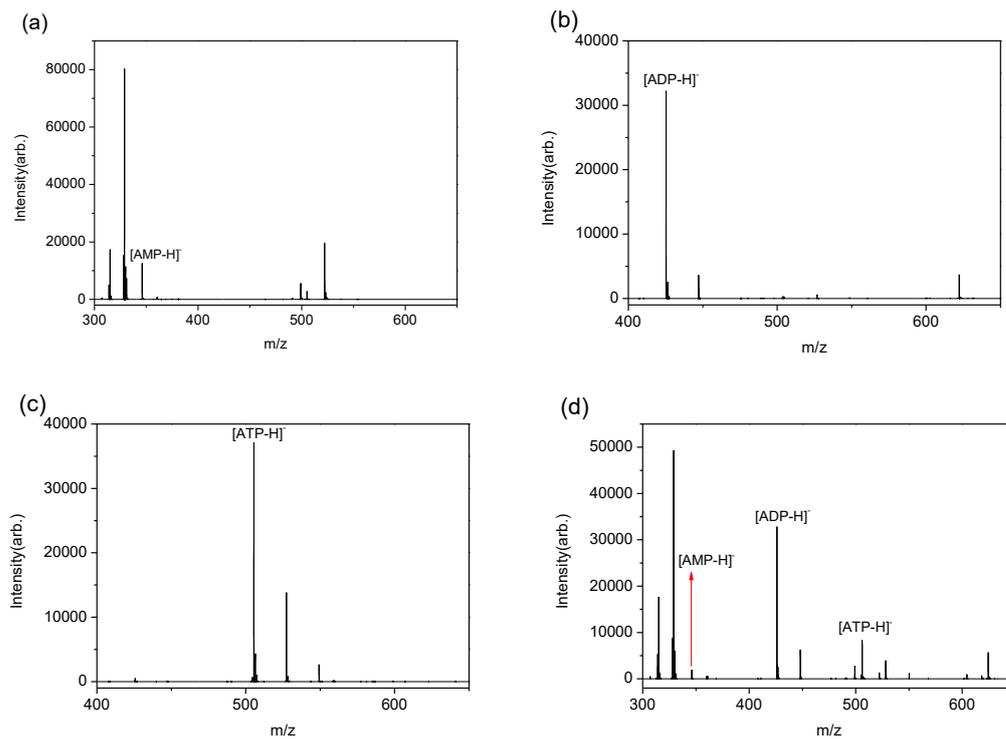
Fig S8. MALDI mass spectra of (a) AMP (1nmol) (b) ADP (1nmol) (c) ATP (1nmol) (d) AMP:ADP:ATP = 1:1:1 (0.33 nmol for each one) with DHBP IL in negative reflectron mode. The molar matrix-to-analyte ratio was approximately 500:1. Laser intensity was 95%. 1000 laser shots randomly distributed in 20 different positions.
