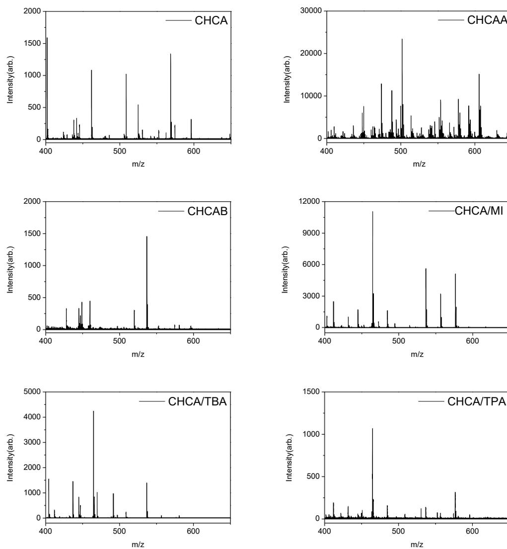
Fig S1. MALDI mass spectra of ATP (1 nmol) in one spot with the matrix of (a) DHB ILs and (b) CHCA ILs in positive reflectron mode. The molar matrix-to-analyte ratio was approximately 500:1. Laser energy was 85% and 65% for each group. 1000 laser shots randomly distributed in 20 different positions.
