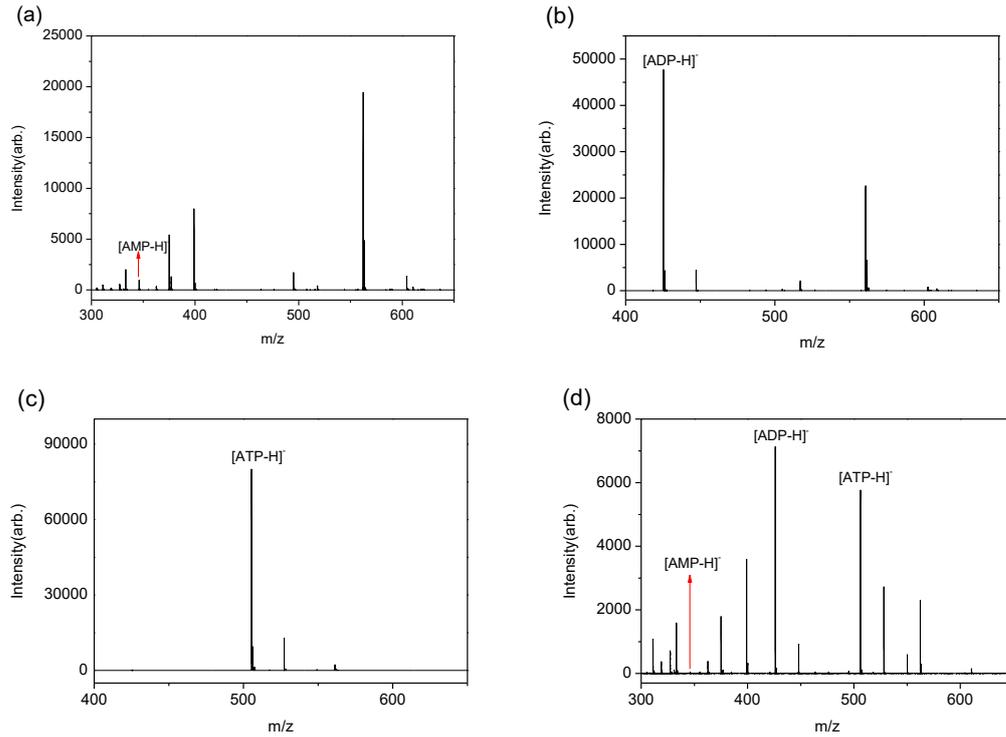
Fig S10. MALDI mass spectra of (a) AMP (1nmol) (b) ADP (1nmol) (c) ATP (1nmol) (d) AMP:ADP:ATP = 1:1:1 (0.33nmol for each one) with CHCA/TPA IL in negative reflectron mode. The molar matrix-to-analyte ratio was approximately 500:1. Laser intensity was 75%. 1000 laser shots randomly distributed in 20 different positions.
