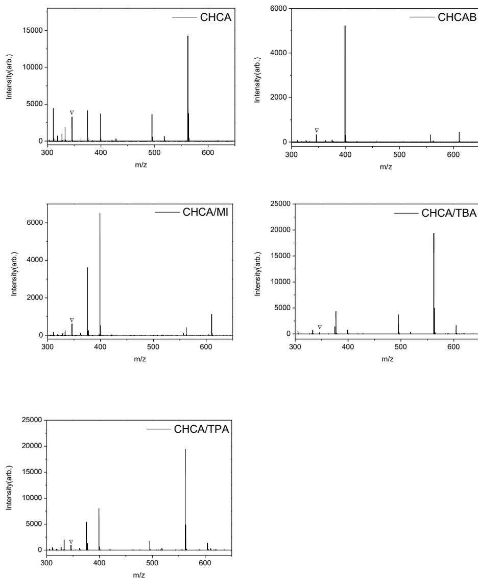
Fig S5. MALDI mass spectra of AMP (1 nmol) in one spot with the matrix of (a) DHB ILs and (b) CHCA ILs in negative reflectron mode. The molar matrix-to-analyte ratio was approximately 500:1. Laser energy was 95% and 75% for each group. 1000 laser shots randomly distributed in 20 different positions.
