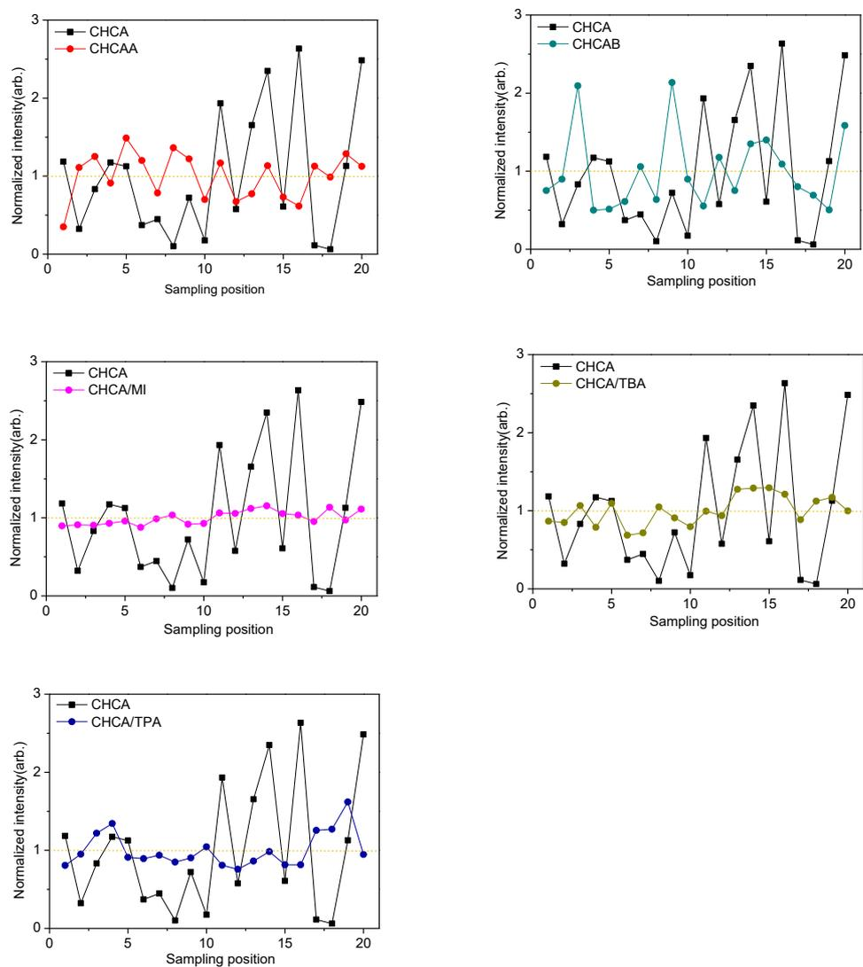
Fig S6. Plot of normalized [ATP-H]<sup>-</sup> signal distribution of (a) DHB ILs and (b) CHCA ILs in 20 different positions of one sample spot on the MALDI metal plate. Laser condition was 1000 shots in one point.
