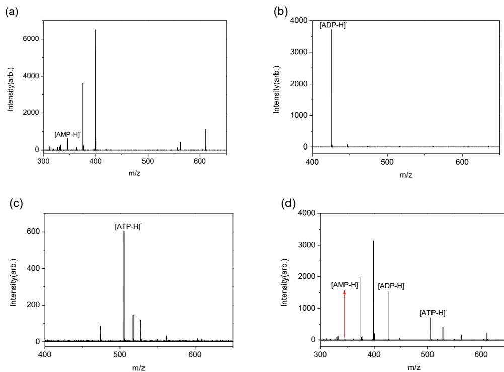
Fig S9. MALDI mass spectra of (a) AMP (1nmol) (b) ADP (1nmol) (c) ATP (1nmol) (d) AMP:ADP:ATP = 1:1:1 (0.33nmol for each one) with CHCA/MI IL in negative reflectron mode. The molar matrix-to-analyte ratio was approximately 500:1. Laser intensity was 75%. 1000 laser shots randomly distributed in 20 different positions.
