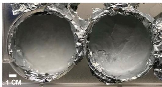
**Figure 3.** Frozen  $\text{CaCl}_2$  on aluminum foil pressed against the interior of the wells of a 6-well plate. Disks were pulled out vertically, ensuring the integrity of frozen  $\text{CaCl}_2$ .
