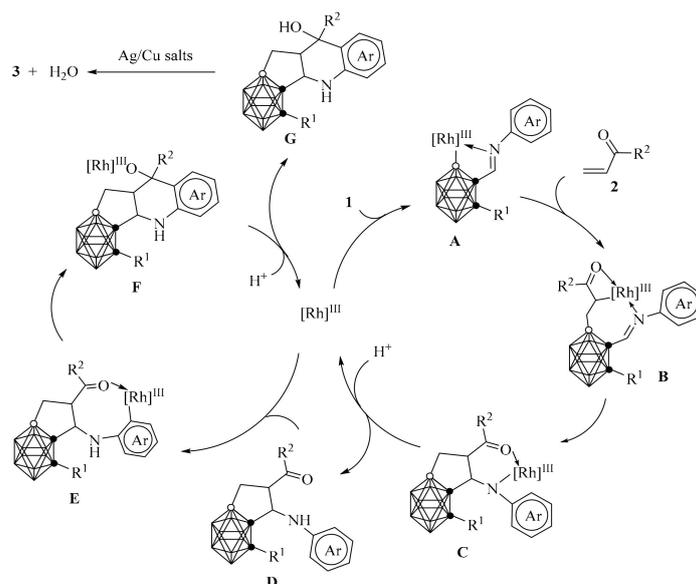
**Scheme 1.** Proposed mechanism for rhodium-catalyzed cascade cyclization of carboranyl *N*-arylimines with vinyl ketones.
