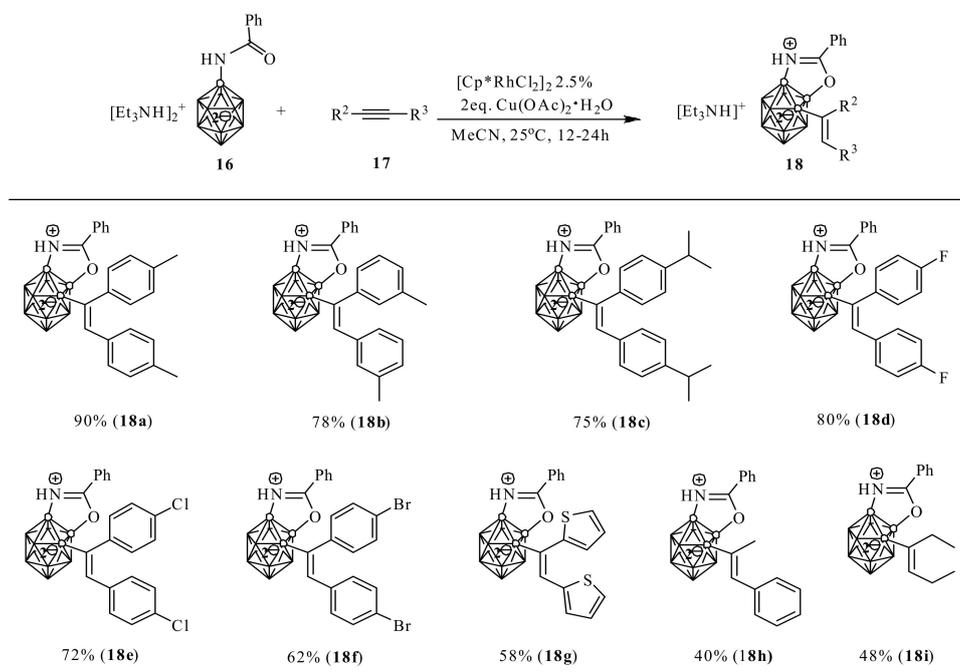
**Figure 6.** Synthesis of dodecaborate-fused oxazoles with amide as directing group.
