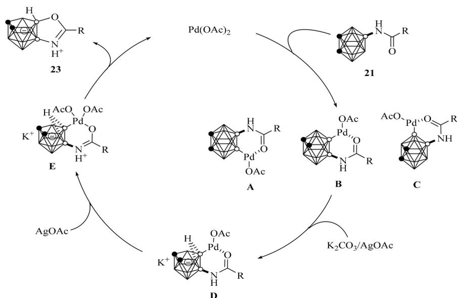
**Scheme 2.** Plausible mechanism for synthesis *nido*-7,8-carborane-fused oxazoles.
