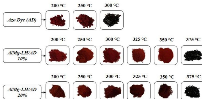
**Figure 11.** Color changes of azo dye, AlMg–LH/AD 10%, and AlMg–LH/AD 20% powders after thermal aging at different temperatures.
