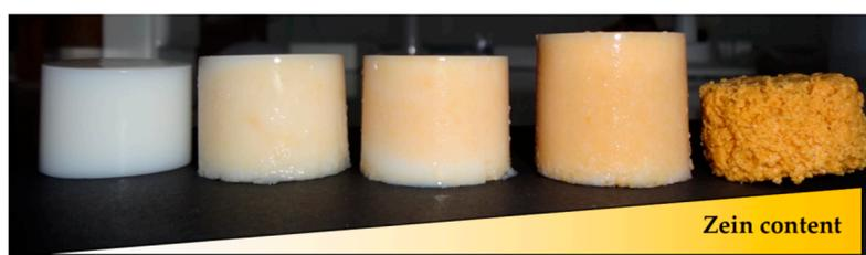
**Figure 1.** Appearance of starch-zein gels obtained from aqueous solutions with 10 wt.% starch and increasing zein content (from left to right, 0:1, 1:5, 1:3, 1:1, and 1:0 zein-to-starch weight ratio).
