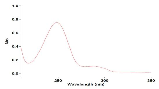
Figure 1. UV-VIS spectroscopy for Phenacetin (internal standard) in the CYP2C11 assay.
