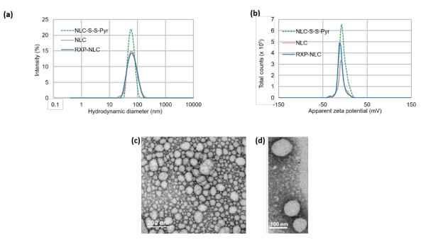
**Figure 2.** Dynamic light scattering (DLS) and SEM characterizations of nanoparticles. (**a**) Size distribution by intensity of NLC-S-S-Pyr, NLC, and RXP-NLC. (**b**) Zeta potential distribution of NLC-S-S-Pyr, NLC, and RXP-NLC. (**c**,**d**) SEM images of NLC-S-S-Pyr after negative staining.
