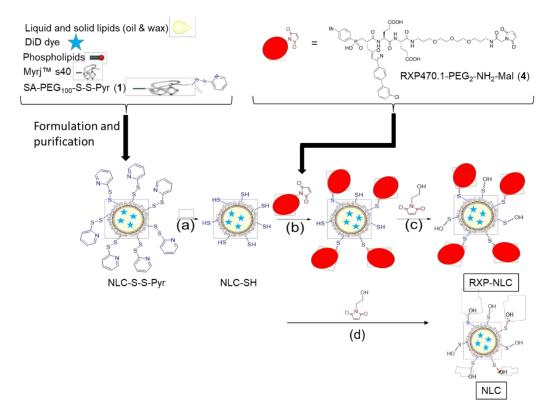
**Figure 1.** Synthesis of RXP470-modified nanostructured lipid carriers (NLC) and control NLC. (a) Addition of dithiothreitol (DTT), incubation 2 h at room temperature, then dialysis overnight. (b) Addition of RXP470.1-maleimide, 4 h incubation at room temperature, then overnight at 4 °C. (c,d) Addition of 1-(2-hydroxyethyl)-1H-pyrrole-2,5-dione, 30 min incubation at room temperature, then dialysis for 24 h.
