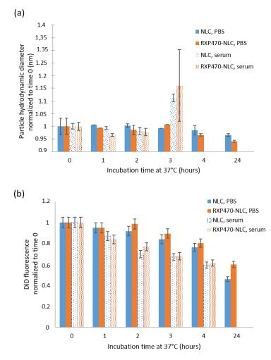
**Figure 3.** NLC and RXP-NLC stability when diluted at 5 mg/mL at 37 °C in 1X PBS buffer or in human serum. (a) Z-average particle diameter (nm) measured by DLS and normalized to value measured just after media and particle mixing. (b) DiD fluorescence (670 nm) normalized to value measured just after media and particle mixing.
