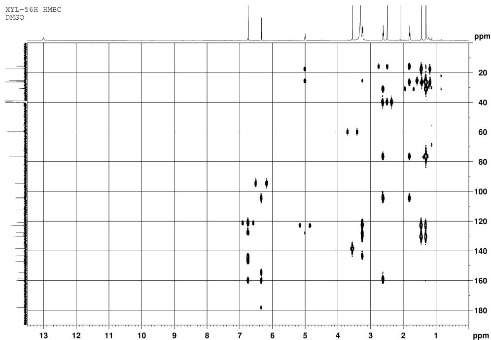
**Figure S16.** HMBC spectrum of compound 4
