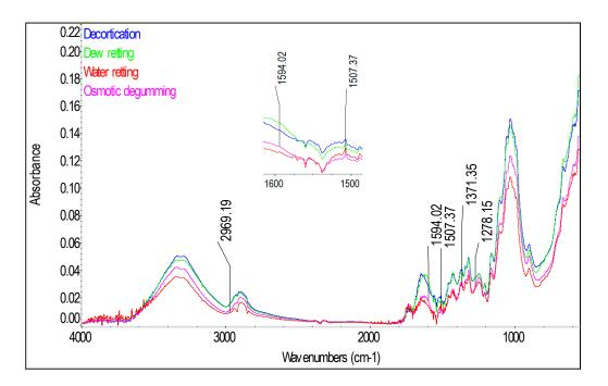
**Figure 9.** The Fourier transform infrared Attenuated Total Reflection spectra of the Białobrzeskie variety, hemp fiber after decortication, dew retting, water retting and osmotically degumming.
