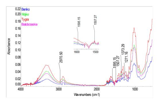
**Figure 8.** The Fourier transform infrared Attenuated Total Reflection spectra of the hemp fibers of Beniko, Wojko, Tygra and Białobrzeskie variety after warm water retting.
