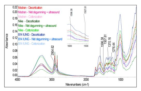
**Figure 7.** The Fourier transform infrared Attenuated Total Reflection spectra of the flax fibers of Modran, Nike and B14 IUNG variety after technological processes.
