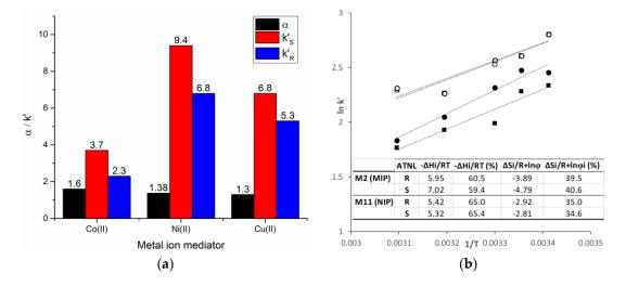
**Figure 4.** (a) Enantioselectivity ( $\alpha$ ) and chromatographic retention (k'<sub>S</sub>/k'<sub>R</sub>) of metal ion-mediated imprinted monoliths (M2—Co(II), M3—Ni(II), M4—Cu(II)). (b) Thermodynamic retention study of ATNL's enantiomers on metal ion-mediated molecularly imprinted (M2,  $\bullet$ —S-ATNL,  $\blacksquare$ —R-ATNL) and non-imprinted (M8,  $\bigcirc$ —S-ATNL,  $\square$ —R-ATNL) polymers.
