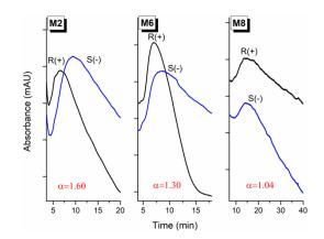
**Figure 3.** Changes in chromatographic selectivity of metal ion-mediated imprinted (M2), non-covalent imprinted (M6) and non-imprinted (M8) monolithic polymer columns. R(+)—R enantiomer of ATNL, S(-)—S enantiomer of ATNL. For chromatographic conditions see footnote of Table 2.
