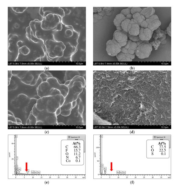
**Figure 2.** Scanning electronmicrographs of monolithic imprinted polymers of M2 (**a**) before and (**b**) after MeOH:AcOH 9:1(v/v) washing, (**c**) M8 and (**d**) M5 before MeOH:AcOH 9:1(v/v) washing. Elemental mapping spectrum of M2 (**e**) before and (**f**) after template removal indicating the washout of the metal pivot ion (Co(II)).
