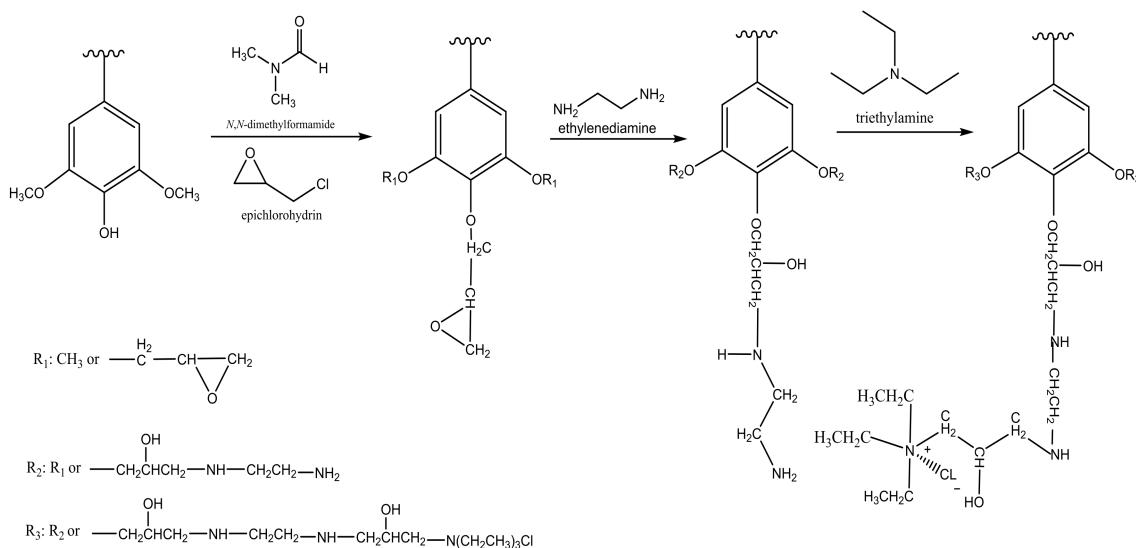
**Figure 2.** Reaction scheme for producing crosslinked amine-based sludge flocculant [34]. The sludge contained mainly lignin and hence the structure of lignin was selected to represent sludge as the raw material in this reaction.
