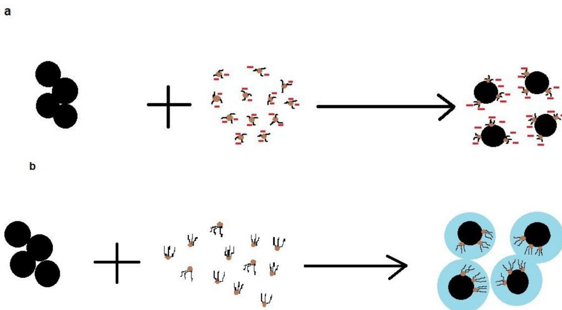
**Figure 5.** Mechanism of dispersants in stabilizing particles in suspensions (a) surface charge density effect and (b) hydrophilicity effect.
