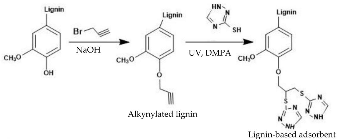
**Figure 4.** Schematic reaction mechanism of thiol-yne alkynylation lignin [69].
