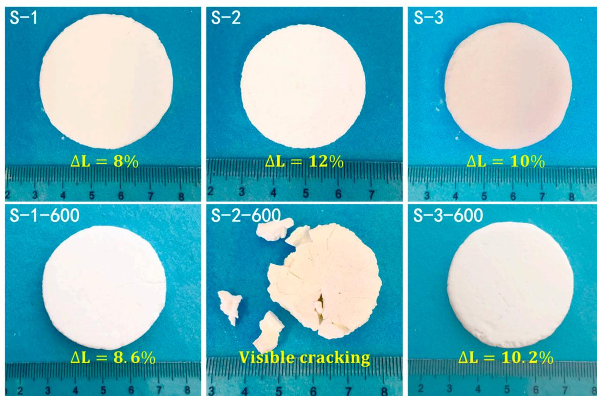
**Figure 3.** Photographs of silica aerogels prepared with different surfactants before and after heat treatment at 600 °C ( $\Delta L$  represents the linear shrinkage of obtained samples).
