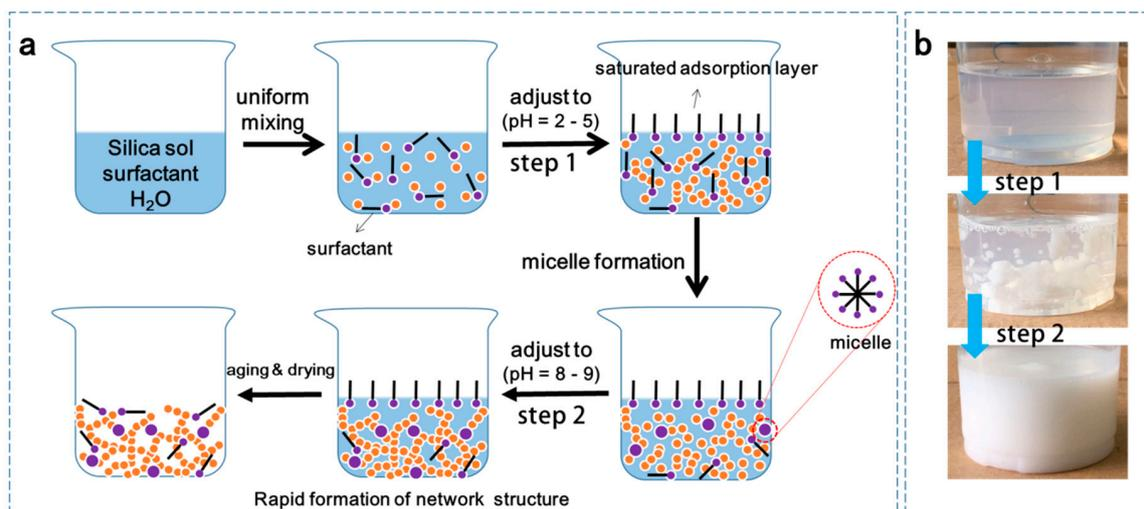
**Figure 1.** (a) Synthesis flowchart of silica aerogels prepared with surfactant. (b) Photographs of the gel evolution during the preparation of silica aerogels with surfactant.
