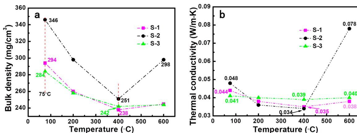
**Figure 2.** (a) Bulk density and (b) room-temperature thermal conductivity of silica aerogels before and after heat treatment at different temperatures.
