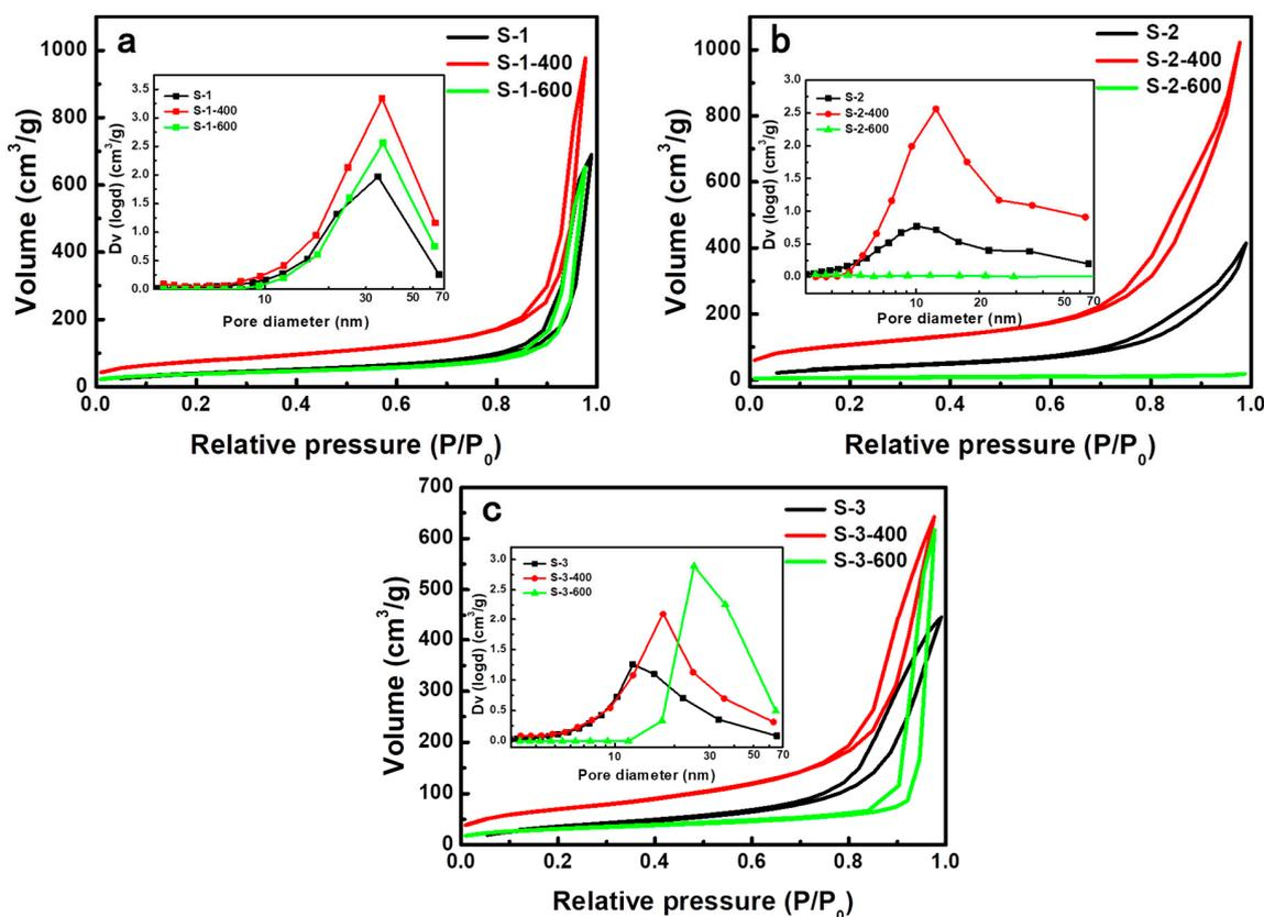
**Figure 7.** N<sub>2</sub> adsorption–desorption isotherms and pore-size distributions of silica aerogels: (a) S-1, (b) S-2 and (c) S-3 before and after heat treatment at 400 °C and 600 °C, respectively.
