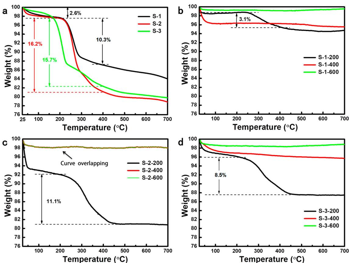
**Figure 6.** Weight loss curves of the silica aerogels: (a) S-1, S-2, and S-3; (b) S-1-200, S-1-400, and S-1-600; (c) S-2-200, S-2-400, and S-2-600, the curve of S-2-600 is almost overlapped with that of S-2-400; (d) S-3-200, S-3-400, and S-3-600.
