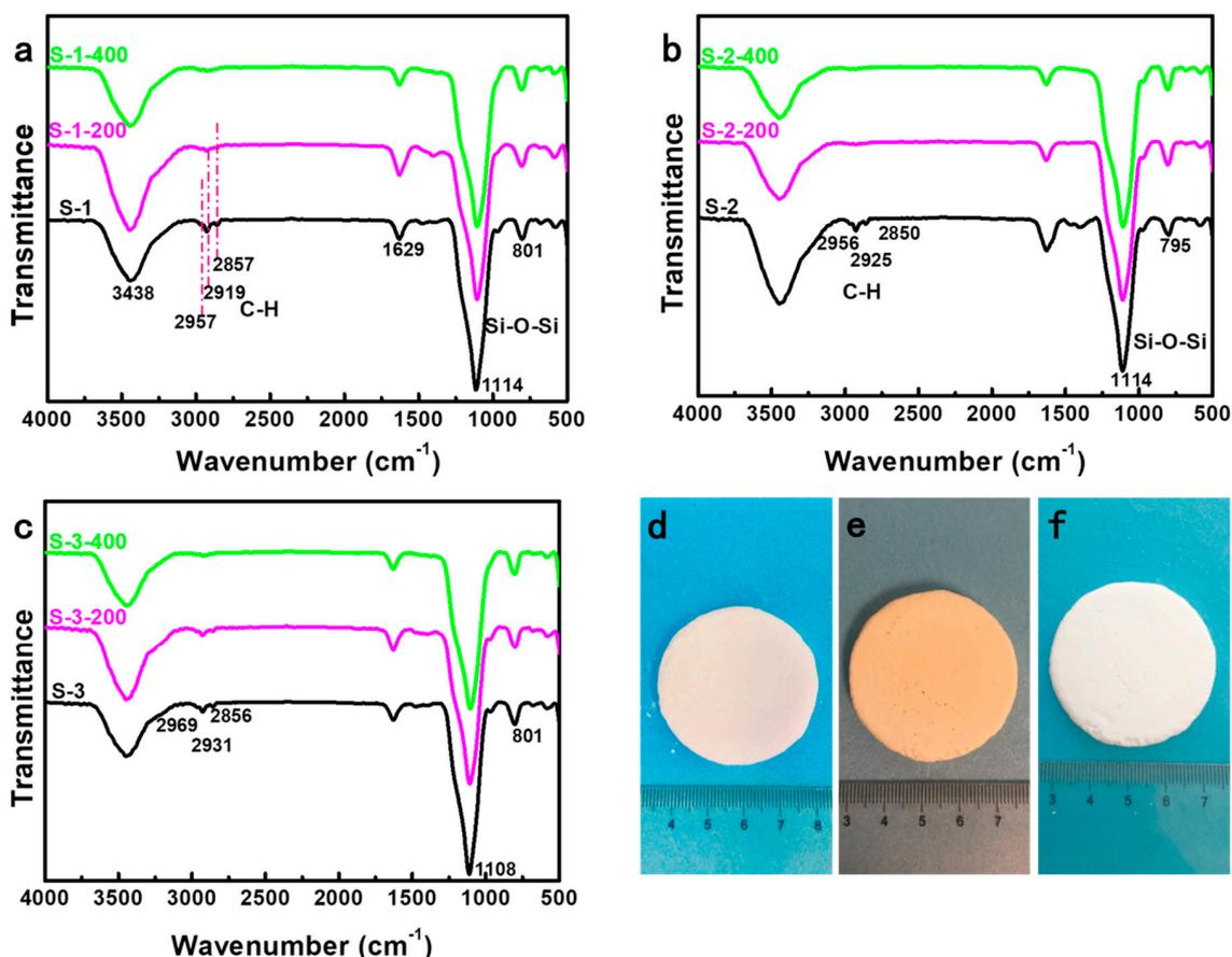
**Figure 5.** FTIR spectra of the silica aerogels: (a) S-1, (b) S-2, and (c) S-3 before and after heat treatment at 200 °C and 400 °C, respectively. (d–f) Representative photographs of silica aerogels prepared with sodium dodecyl sulfate (SDS) before and after heat treatment at 200 °C and 400 °C, respectively.
