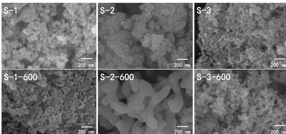
**Figure 4.** SEM images of silica aerogels prepared with different surfactants before and after heat treatment at 600 °C.
