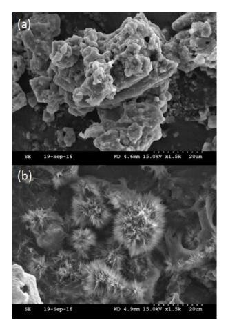
Figure 2. FE-SEM images of Fe<sub>3</sub>O<sub>4</sub>/MIPs (a) and DES-7-Fe<sub>3</sub>O<sub>4</sub>/MIPs (b).
