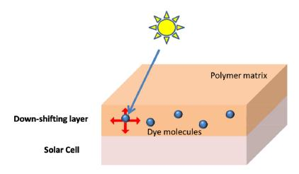
Figure 2. Structure of a typical luminescent down-shifting layer.
