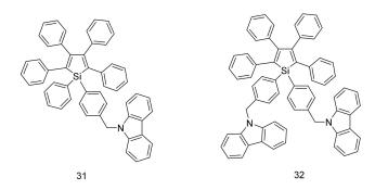
Figure 10. Structures of hexaphenylsilole molecules used as donors in OPV.
