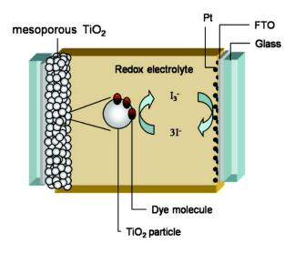
**Figure 7.** Schematic of a typical dye-sensitized solar cell (DSSC). (reprinted with permission from ref. [27], Copyright 2010 American Chemical Society).
