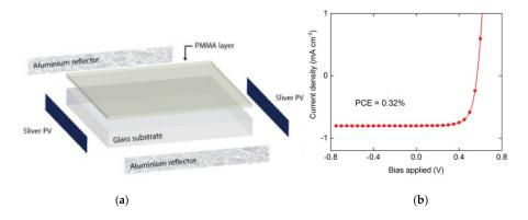
**Figure 6.** (a) Structure of the LDS device; (b) Current-voltage characteristics of a transparent planar concentrator device fabricated using 15. (reprinted with permission from ref. [4], Copyright 2017 American Chemical Society).
