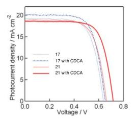
**Figure 8.** Current density vs. voltage characteristics for DSSCs with indoline dyes 17 and 21 as sensitizers with/without chenodeoxycholic acid (CDCA) under AM1.5 simulated sunlight ( $100 \text{ mW cm}^{-2}$ ) illumination. (reprinted with permission from ref. [32], Copyright 2008 Royal Society of Chemistry).
