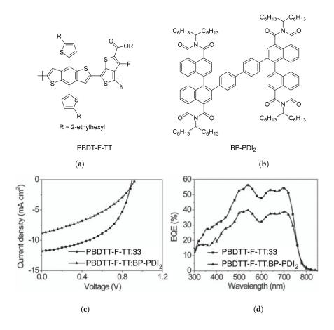
**Figure 11.** (a) Chemical structure of polymer donor PBDTT-F-TT; (b) Chemical structure of biphenyl-bridged perylene diimide dimer (BP-PDI<sub>2</sub>); (c) current-voltage characteristics of bulk heterojunction (BHJ) solar cells fabricated from PBDTT-F-TT:33 and PBDTT-F-TT:BP-PDI<sub>2</sub> under AM1.5 irradiation at 100 mW cm<sup>-2</sup>; (d) External quantum efficiency spectra of the devices. (reprinted with permission from ref. [42]. Copyright 2015 Wiley-VCH).
