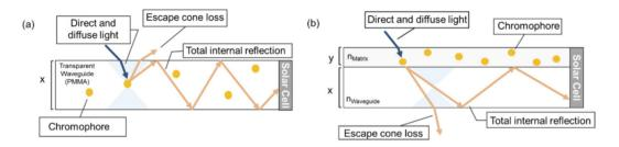
**Figure 4.** Conventional structures for luminescent solar concentrator (LSC) applications: (**a**) millimeter-thick waveguides infused with fluorescent dyes; (**b**) micron-thick thin layer matrices cast on top of a waveguide. (reprinted with permission from ref. [22], Copyright 2014 Nature Publishing Group).
