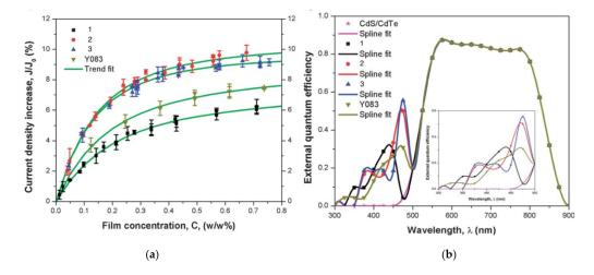
**Figure 3.** (a) The increase of short circuit current density ( $J_{sc}$ ) vs. the different concentrations of the LDS film placed on the CdTe solar cell surface for fluorophores 1–3 and Y083; (b) The enhanced spectral response at short-wavelengths after the LDS film was placed on the CdTe solar cell surface for fluorophores 1–3 and Y083. (reprinted with permission from ref. [17], Copyright 2013 Royal Society of Chemistry).
