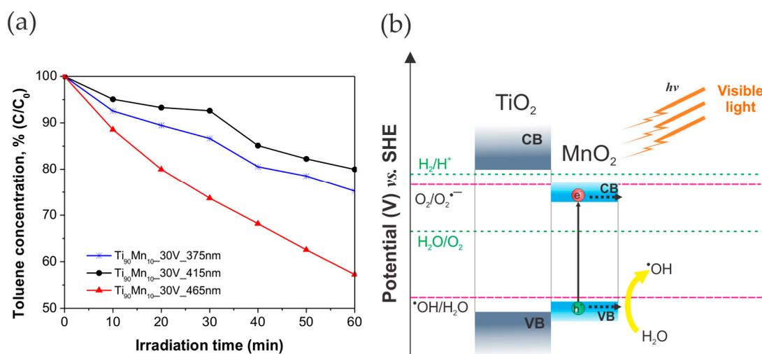
**Figure 8.** (a) Photoactivity of  $\text{Ti}_{90}\text{Mn}_{10}\text{-30V}$  sample in gas phase degradation of toluene under different wavelengths of irradiation ( $\lambda_{\text{max}} = 375, 415, 465 \text{ nm}$ ) and (b) possible excitation mechanism of  $\text{TiO}_2\text{-MnO}_2$  NTs under Vis light irradiation.
