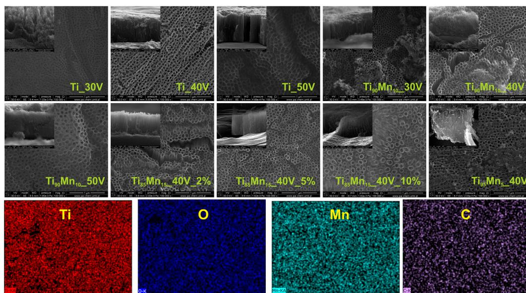
**Figure 1.** Top-view and cross-sectional SEM images of pristine  $\text{TiO}_2$  and  $\text{TiO}_2\text{-MnO}_2$  NTs (the effect of applied voltage, manganese content in the Mn/Ti alloy, and water content in the electrolyte on the morphology of formed nanotubes) and EDX mapping of the  $\text{Ti}_{90}\text{Mn}_{10}$ \_30V sample.
