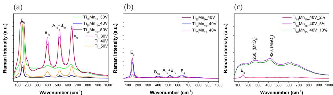
**Figure 4.** Raman spectra of pristine  $\text{TiO}_2$  and  $\text{TiO}_2\text{-MnO}_2$  NTs. Effect of (a) anodization potential; (b) manganese content in the alloy; and (c) water content in the electrolyte.
