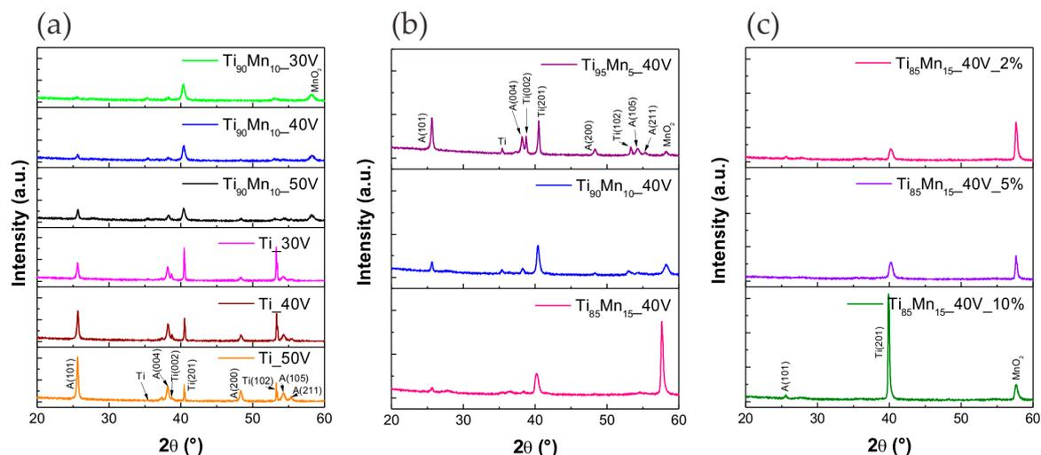
**Figure 3.** XRD spectra of pristine  $\text{TiO}_2$  and  $\text{TiO}_2$ – $\text{MnO}_2$  NTs. Effect of (a) anodization potential; (b) manganese content in the alloy; and (c) water content in the electrolyte.
