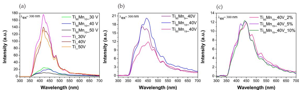
**Figure 6.** Photoluminescence spectra of pristine  $\text{TiO}_2$  and  $\text{TiO}_2\text{-MnO}_2$  NTs. Effect of (a) anodization potential; (b) manganese content in the alloy; and (c) water content in the electrolyte.
