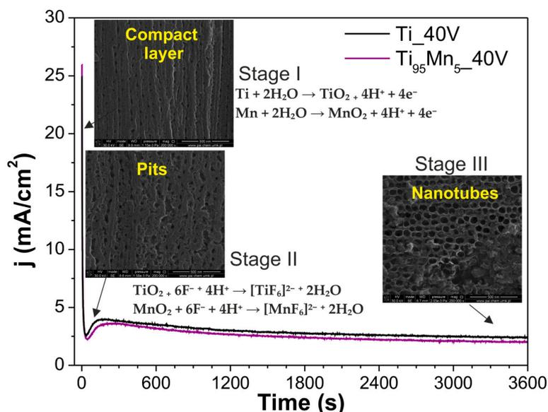
Figure 2. Proposed growth mechanism of  $\text{TiO}_2$ – $\text{MnO}_2$  NTs.
