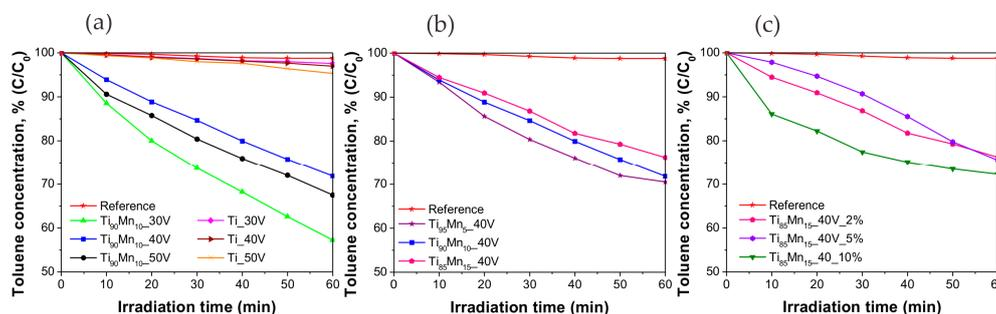
**Figure 7.** Photoactivity of pristine  $\text{TiO}_2$  and  $\text{TiO}_2\text{-MnO}_2$  NTs in gas phase degradation of toluene under Vis light irradiation ( $\lambda_{\max} = 465$  nm). Effect of (a) applied voltage; (b) manganese content in the alloy, and (c) water content in the electrolyte.
