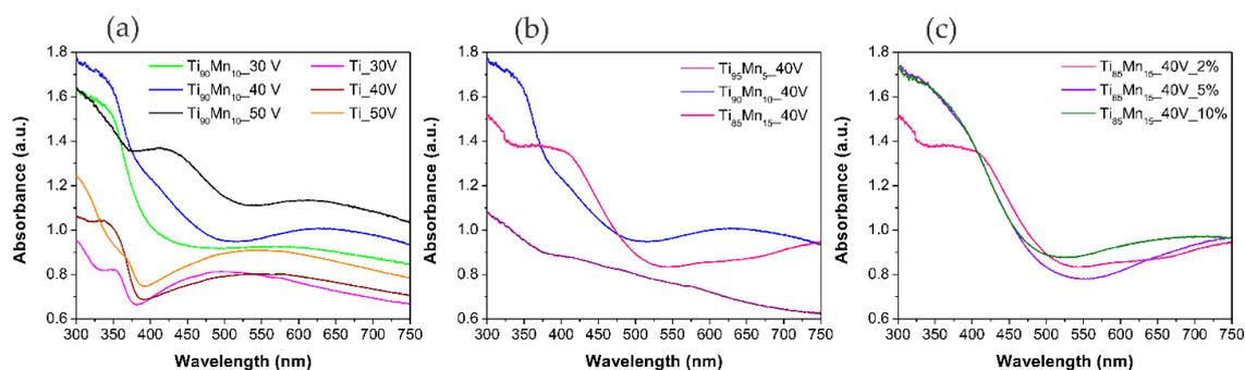
**Figure 5.** UV-Vis spectra of pristine  $\text{TiO}_2$  and  $\text{TiO}_2\text{-MnO}_2$  NTs. Effect of (a) anodization potential; (b) manganese content in the alloy; and (c) water content in the electrolyte.
