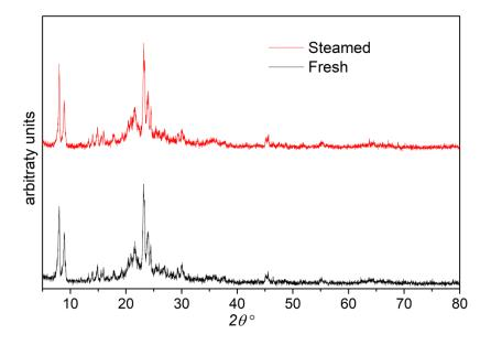
Figure S2. XRD patterns of the fresh-calcined and steamed (at 770°C, 7 hrs, 50% steam/He) P/ZSM-5 additive.
