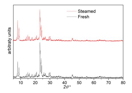
Figure S1. XRD patterns of fresh and steamed (at 770°C, 7 hrs, 50% steam/He) P/H-ZSM-5 zeolites
