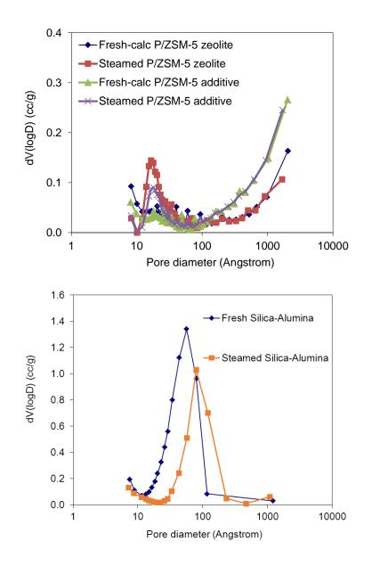
**Figure S3.** Pore size distribution curves based on the BJH analysis of the N<sub>2</sub> adsorption data of freshcalcined and steamed P/H-ZSM-5 pure zeolite, P/ZSM-5 additive and silica-alumina; steaming conditions were 770°C, 7 hrs, 50% steam/He.
