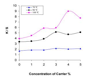
Figure 2. Effect of the concentration of carrier on the dyeing for disperse dye 3b at different dyeing temperatures.
