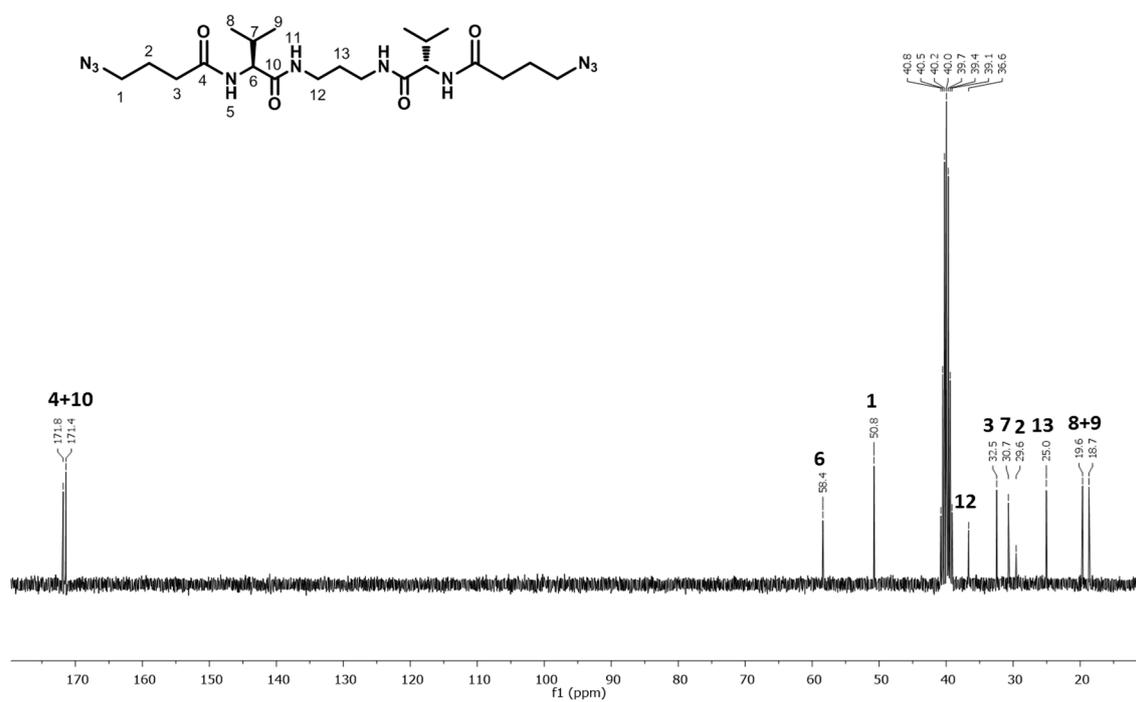
**Figure S5.**  $^{13}\text{C-NMR}$  spectrum of compound IV (DMSO- $d_6$ , 300 MHz).
