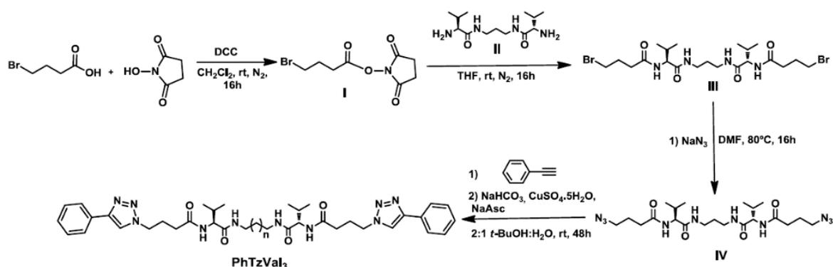
Figure S1. Scheme for the synthesis of PhTzVal<sub>3</sub> gelators.
