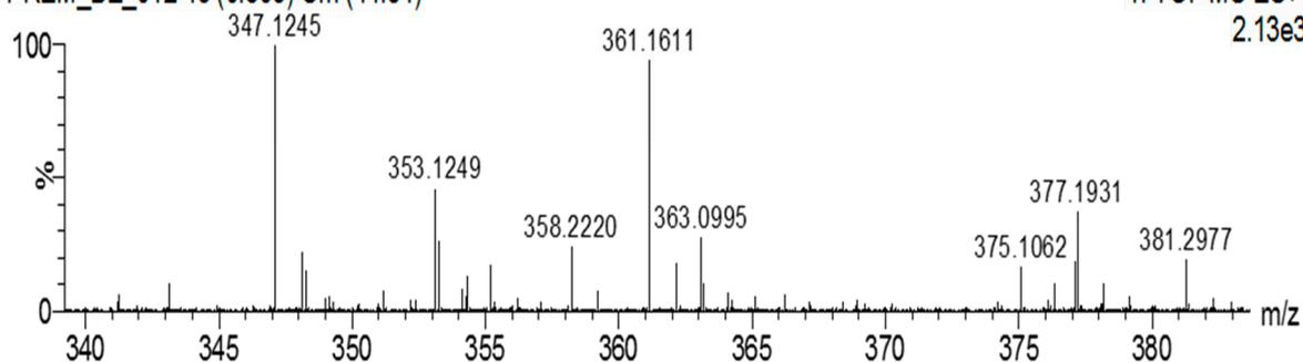
**Figure S11.** High-resolution mass spectrometry of the final product, isolated by type II alumina column chromatography of the crude belonging to the three component reaction carried for 2 days in the presence of 10 mol %  $\text{Cu(I)-PhTzVal}_3$ .
