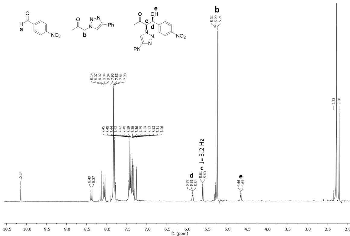
**Figure S10.** Typical  $^1\text{H-NMR}$  spectrum of a catalytic reaction in the presence of 10 mol%  $\text{Cu(I)-PhTzVal}_3$  ( $\text{CDCl}_3$ , 300 MHz).
