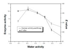
**Figure 5.** Effect of water activity on the enzymatic esterification of ibuprofen. Reaction conditions: the reactions were carried out in *n*-heptane (10 mL) with racemic ibuprofen (0.2 mmol), 1-octanol (0.2 mmol) and the immobilized APE1547 powder (160 mg) at 45 °C. The ultrasound power was 225 W.
