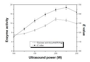
**Figure 3.** Effect of ultrasound power on the enzymatic esterification of ibuprofen. Reaction conditions: the reactions were carried out in *n*-heptane (10 mL,  $a_w$  0.21) with racemic ibuprofen (0.2 mmol), 1-octanol (0.2 mmol) and the immobilized APE1547 powder (160 mg) at 45 °C.
