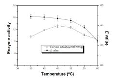
**Figure 4.** Effects of temperature on the enzymatic esterification of ibuprofen. Reaction conditions: the reactions were carried out in *n*-heptane (10 mL,  $a_w$  0.21) with racemic ibuprofen (0.2 mmol), 1-octanol (0.2 mmol) and the immobilized APE1547 powder (160 mg) at different temperature. The ultrasound power was 225 W.
