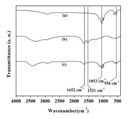
**Figure 2.** The FTIR spectrum of  $Cu_3(PO_4)_2$  matrices (curve a), APE1547 (curve b) and the immobilized APE1547 (curve c).
