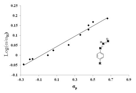
**Figure S1.** Plot of the logarithm of the global electrophilicity ratios of substituted azides versus the  $\sigma_P$  Hammett substituent constants. The value of the regression coefficient for the least-squares fit to a linear plot is  $R^2 = 0.97$ .
