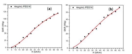
**Figure S5.** SAR values of Fe<sub>3</sub>O<sub>4</sub> MNPs synthesized in (**a**) PEG 200 and (**b**) EG as a function of AC field amplitudes and at a frequency of 355 kHz. The Fe<sub>3</sub>O<sub>4</sub> MNPs are dispersed in soft solid PEG1000 and the hyperthermia measurements have been performed starting with room temperature up to 37 °C. The data are fitted with a sigmoidal function (red lines).
