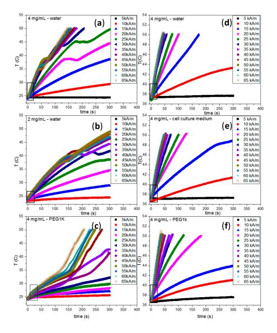
**Figure S4.** Heating curves of large Fe<sub>3</sub>O<sub>4</sub> MNPs dispersed in different media and recorded starting with room temperatures (left panels: **a**–**c**) and 37 °C (right panels: **d**–**f**) as a function of AC magnetic field amplitudes at 355 kHz. The black rectangles frame the slope ( $\Delta T/\Delta t$ ) used in SAR determination.
