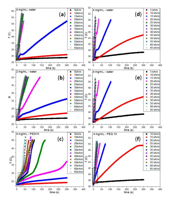
**Figure S3.** Heating curves of small Fe<sub>3</sub>O<sub>4</sub> MNPs dispersed in different media and recorded starting with room temperatures (left panels:  $\mathbf{a}$ - $\mathbf{c}$ ) and 37 °C (right panels:  $\mathbf{d}$ - $\mathbf{f}$ ) as a function of AC magnetic field amplitudes at 355 kHz. The black rectangles frame the slope ( $\Delta T/\Delta t$ ) used in SAR determination.
