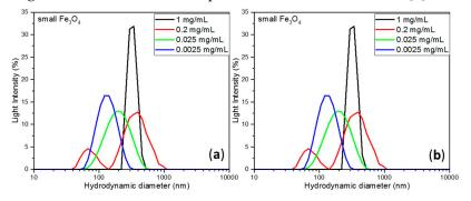
Figure S1. Hydrodynamic diameter of small (a) and large (b) Fe<sub>3</sub>O<sub>4</sub> MNPs as a function of the concentration.
