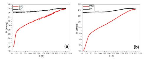
**Figure S2.** ZFC and FC magnetization curves of (**a**) small and (**b**) large Fe<sub>3</sub>O<sub>4</sub> MNPs, acquired in an external magnetic field of 50 mT.
