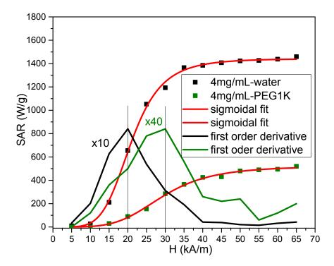
**Figure S6.** The SAR values of small Fe<sub>3</sub>O<sub>4</sub> MNPs as a function of AC field amplitudes in water and PEG1K. The experimental results have been fitted with a sigmoidal function (red lines). The first-order derivatives of the experimental data were multiplied by 10 and 40 for clarity (black and green lines). The maxima in first-order derivative correspond to the inflection points of sigmoidal function and give the values of H<sub>cHyp</sub>.
