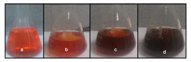
**Figure 1.** Synthesis of silver nanoparticles (Ag-NPs) using aqueous extract of *sumac*: (**a**) aqueous extract of *sumac*; (**b**) initial point of time; (**c**) mid-point of time and (**d**) final point of time.
