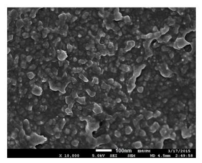
Figure 5. Field emission scanning electron microscopy (FESEM) image of Ag-NPs synthesized using *sumac* extract.
