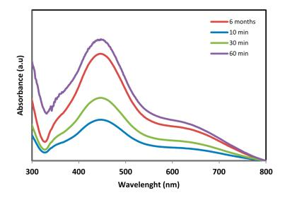
Figure 2. UV-visible spectra of bio-synthesized Ag-NPs.
