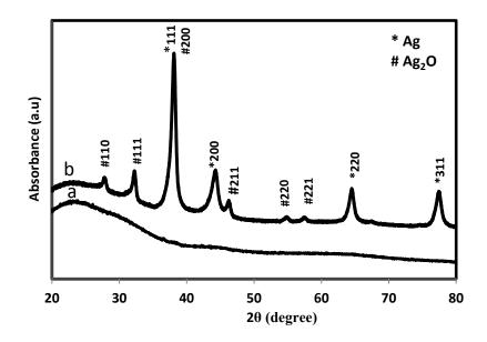
Figure 3. XRD pattern of *Sumac* (a) and bio-formed NPs (b).
