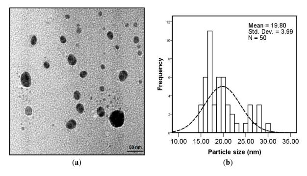
Figure 4. TEM image (a) and particle size distributions (b) of bio-synthesized nanoparticles.
