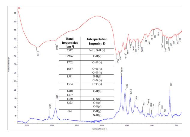
Figure S8. Raman and IR spectra of 8 (impurity D).
