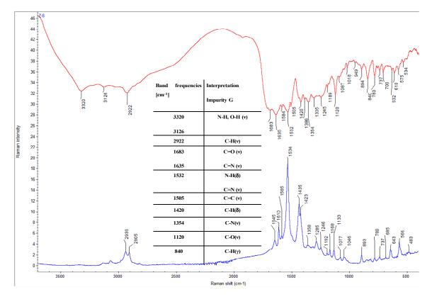
Figure S7. Raman and IR spectra of 7 (impurity G).
