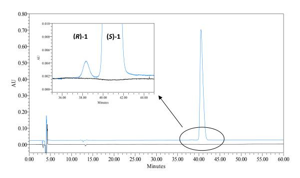
**Figure S1.** Chromatogram for the test for enantiomeric purity of Pemetrexed Disodium. *(S)*-1—Pemetrexed Disodium; *(R)*-1—enantiomeric impurity.
