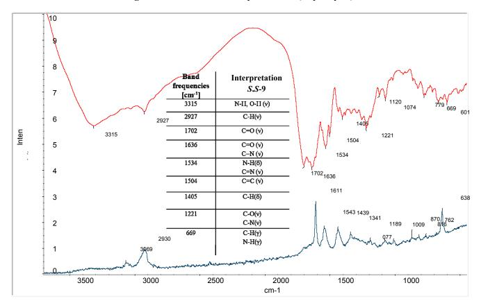
Figure S9. Raman and IR spectra of *S*,*S*-9.
