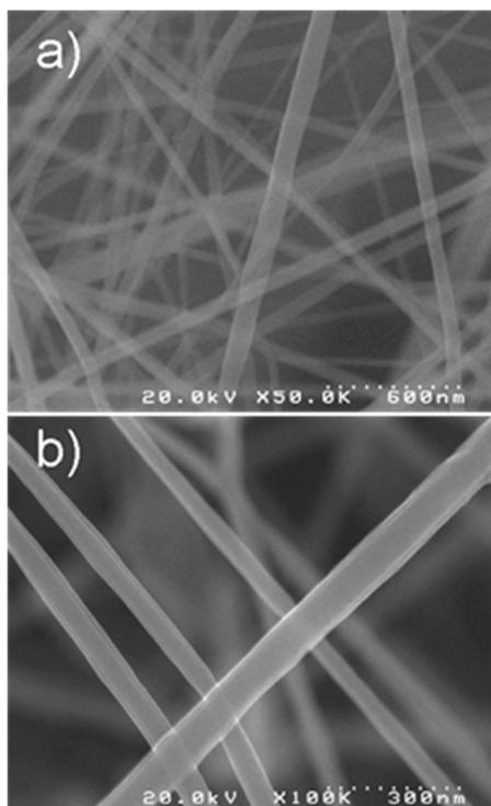
**Figure 1.** (a) Pulp cellulose-ESNW (scale bar, 600 nm); (b) Cotton cellulose-ESNW (scale bar, 300 nm). Reproduced from [44] with permission of SAGE Publications, Ltd.
