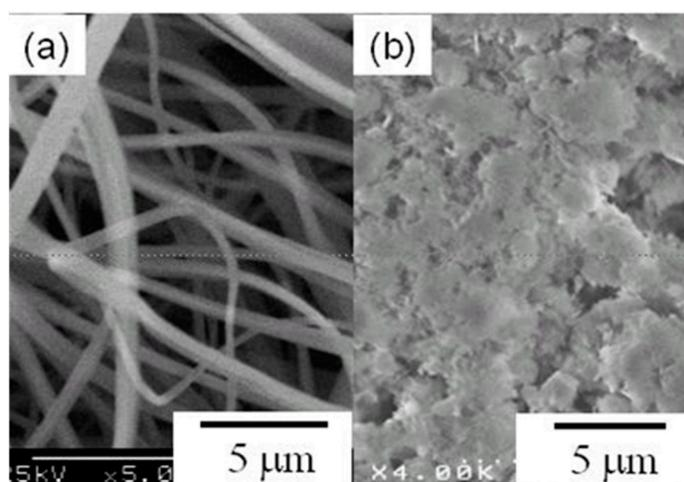
**Figure 4.** (a) Scanning electron microscopy of a Cellulose-copoly [Ser(PO<sub>3</sub>H<sub>2</sub>)<sup>x</sup>, Asp<sup>y</sup>]-Composite-ESNW ( $x:y = 75:25$ ) (1.0 wt % towards cellulose); (b) Morphology of hydroxyapatite after *in vitro* calcium phosphate deposition, which entirely covers the ESNW matrix.
