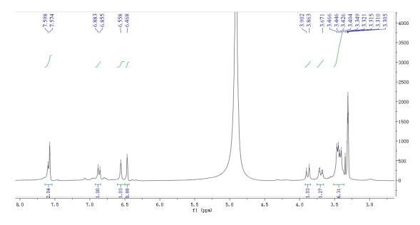
Figure S11. <sup>1</sup>H-NMR spectrum of 2 in CD<sub>3</sub>OD.
