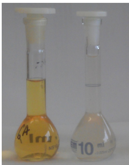
Figure S44. Photograph of the Fe(II) cylinder 6a obtained at 10^{-4} M concentrations before (left) and after the addition of histidine (right) in acetonitrile.
